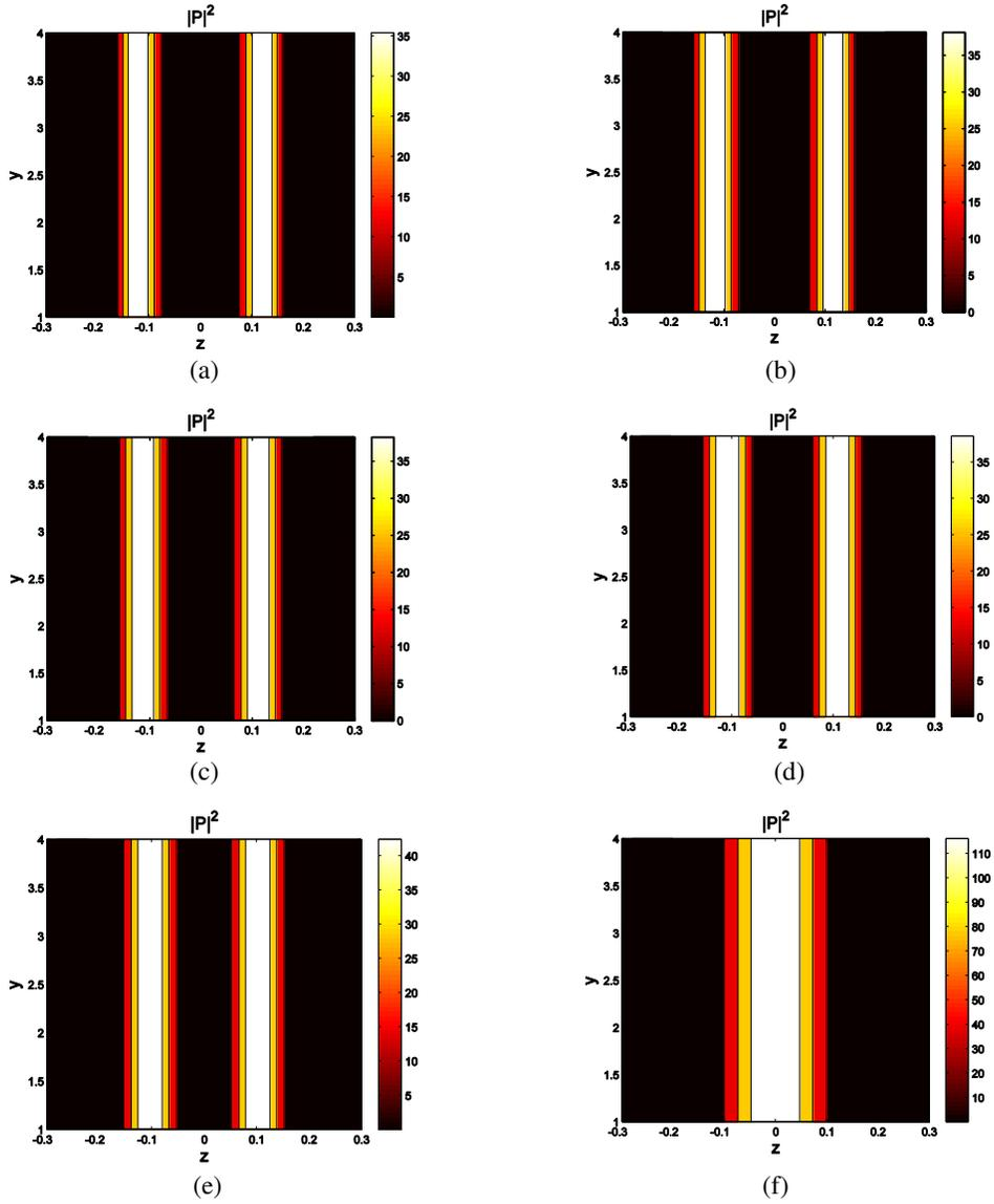
**Figure 4.** Power along the guide for  $d_1 = 0.2$  and at (a)  $D = 1.1$ , (b)  $D = 1.3$ , (c)  $D = 1.5$ , (d)  $D = 1.7$ , (e)  $D = 1.9$ , (f)  $D = 2$  and  $m = 0$ .
