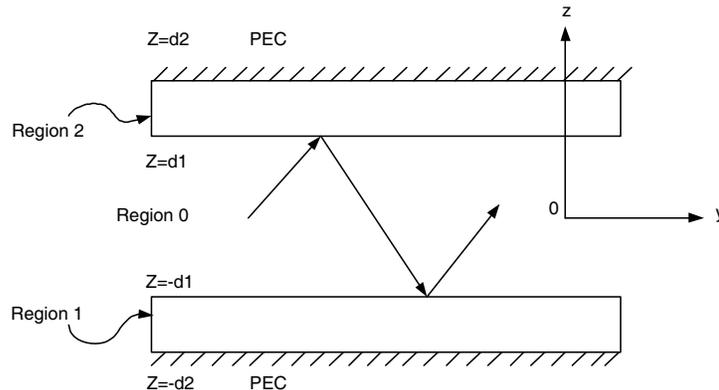
**Figure 1.** Three layered fractal waveguide.
