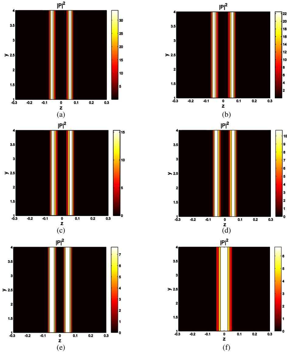
**Figure 2.** Power along the guide for  $d_1 = 0.1$  and at (a)  $D = 1.1$ , (b)  $D = 1.3$ , (c)  $D = 1.5$ , (d)  $D = 1.7$ , (e)  $D = 1.9$ , (f)  $D = 2$  and  $m = 0$ .
