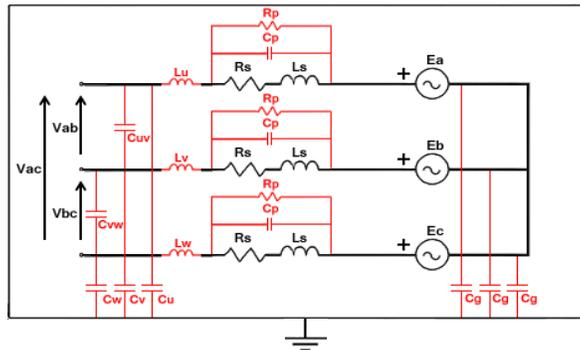
**Figure 5.** Circuit model of the PMSM. The external black rectangle represents the metallic chassis, black circuit elements pertain to the functional low-frequency model, whereas red circuit elements describe high-frequency parasitic components.
