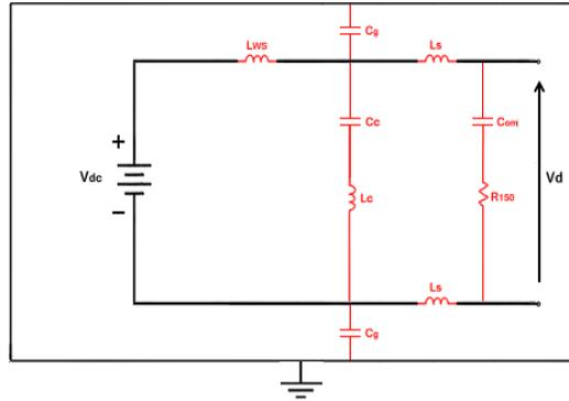
**Figure 6.** Circuit model of the battery. The external black rectangle represents the metallic chassis, black circuit elements pertain to the functional low-frequency model, whereas red circuit elements describe behavioral components modeling the high-frequency response.
