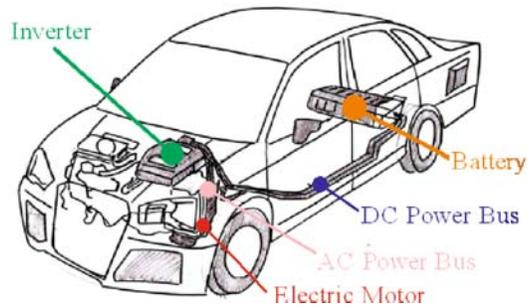
**Figure 1.** General layout of the electric-vehicle powertrain.
