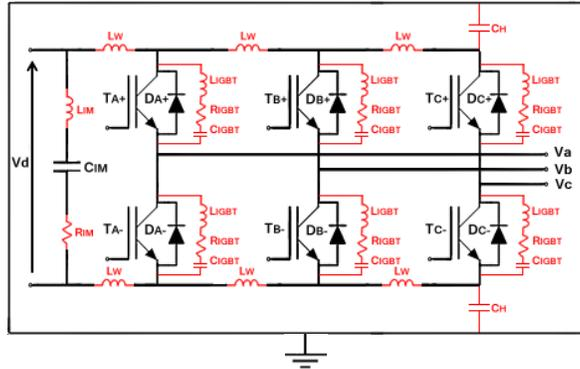
**Figure 4.** Circuit model of the inverter. The external black rectangle represents the metallic chassis, black circuit elements pertain to the functional low-frequency model, whereas red circuit elements describe high-frequency parasitic components.
