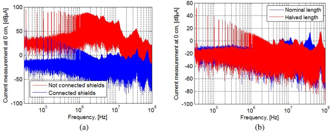
**Figure 12.** CE at the nominal operating condition of the powertrain (CISPR current-probe method): (a) Comparison of a test setup with proper grounding of cable shields, and a setup lacking ground connections; (b) Comparison of a test setup with nominal length of the dc power bus and a setup with halved length.
