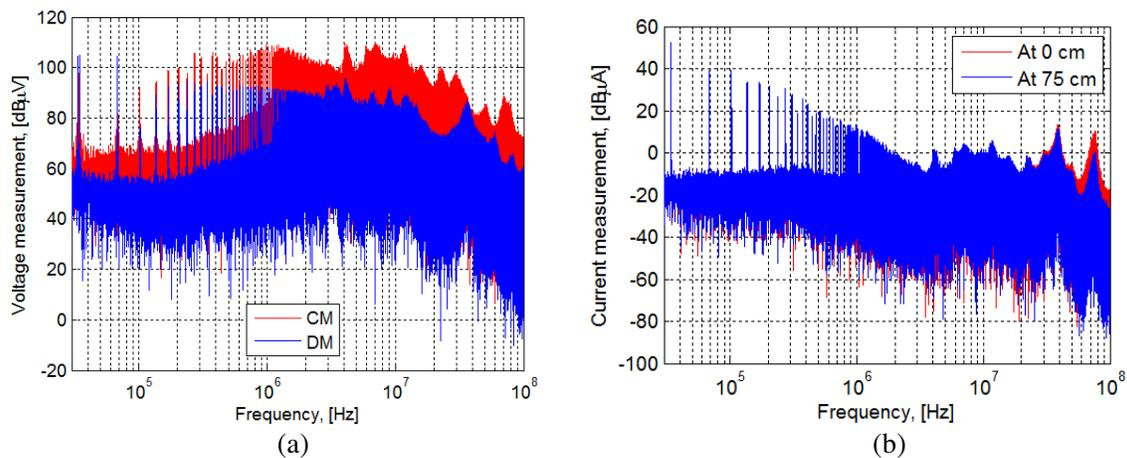
**Figure 11.** CE evaluated at the nominal operating condition of the powertrain: (a) CISPR voltage method with modal decomposition, (b) CISPR current-probe method at two different positions from the inverter.
