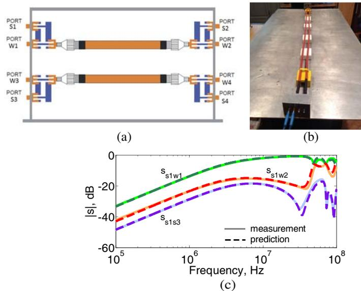
**Figure 9.** (a) Principle drawing and (b) picture of the experimental test setup for the characterization of power-bus scattering parameters. (c) Comparison of selected measurements versus predictions.
