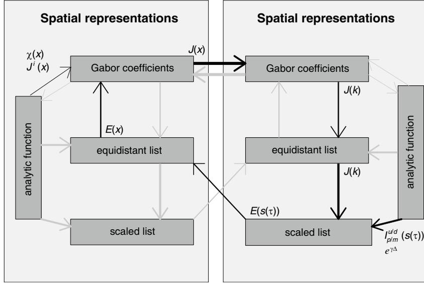
**Figure 5.** The various transformations and representations we have explained in Section 4. The thickness of the arrows signifies the speed of the transformation qualitatively. Thicker means faster. The black arrows signify the different transformations that are actually used in the algorithm, the grey ones are possible, but not used.
