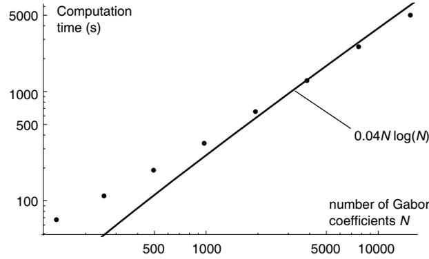
**Figure 11.** Dots indicate computation time of one matrix vector product of operator  $A$  versus the number of Gabor coefficients for an increasing number of modulation frequencies in the Gabor frame. Solid line indicates a reference of  $O(N \log N)$  behaviour.
