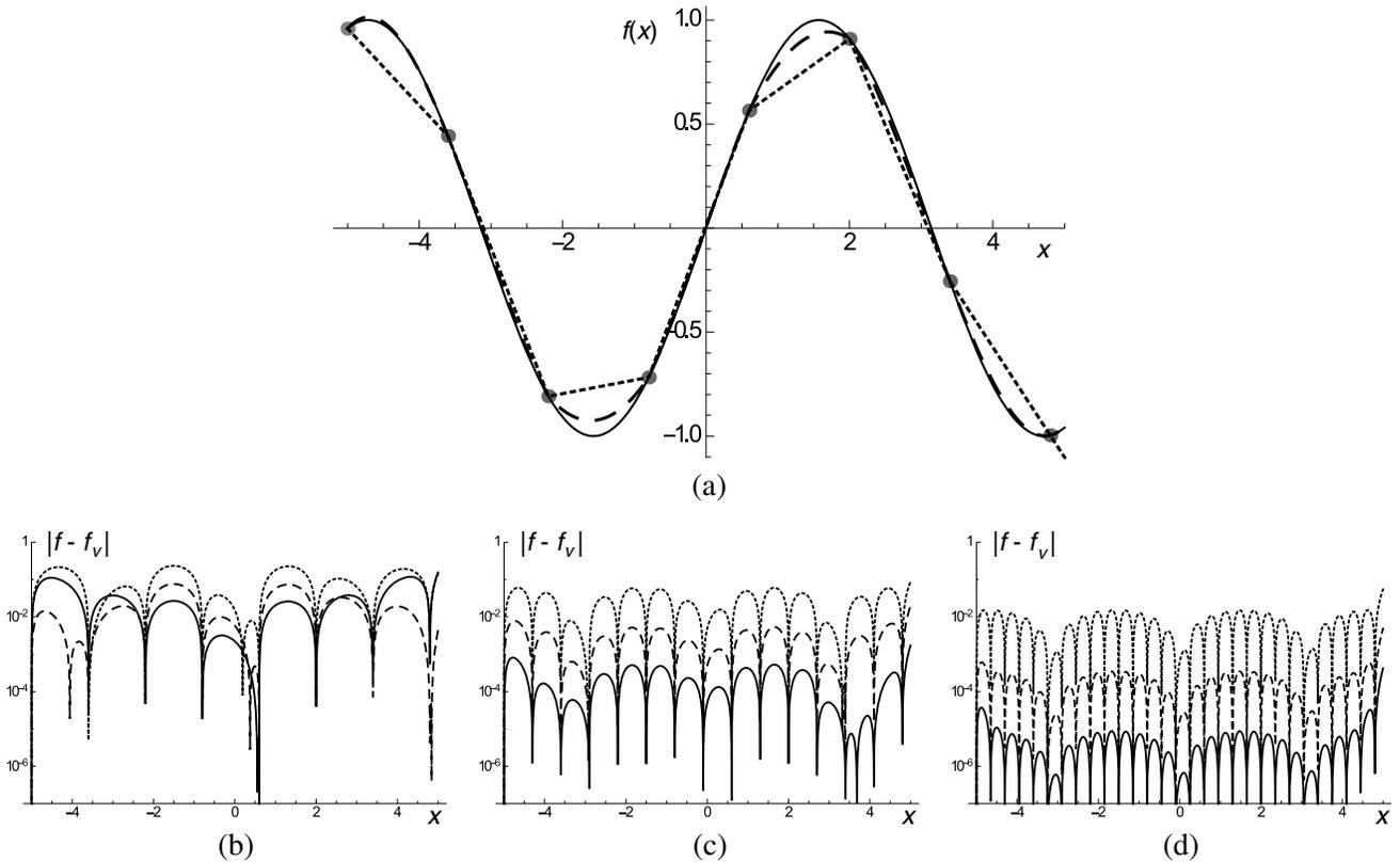
**Figure 4.** (a) Solid line:  $f_V(x)$  a sine function as validation. Dotted: A linear interpolation  $f$  of the validation  $f_V$ , dashed: A third order Hermite spline interpolation  $f$  of the validation  $f_V$ . (b) The absolute error of the approximations  $|f(x) - f_V(x)|$ : linear interpolation (dotted), 3rd order Hermite interpolation (dashed), 5th order Hermite interpolation (solid). (c) The same for double sampling. (d) The same for quadruple sampling.
