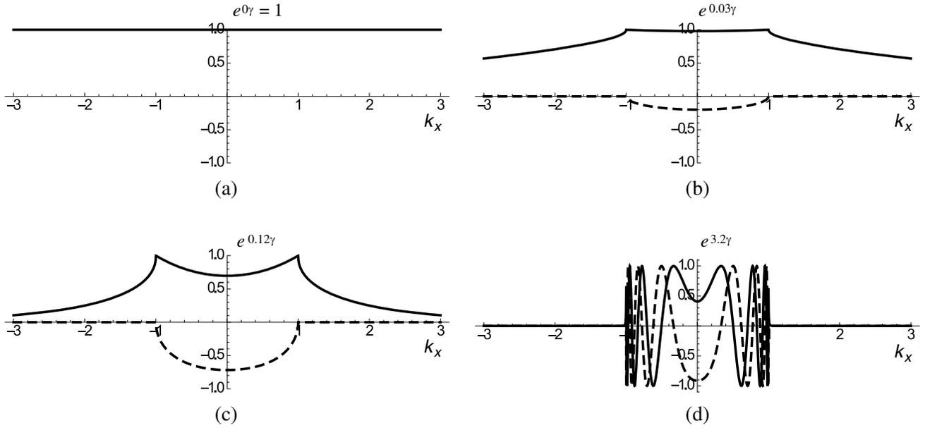
**Figure 2.** The spectrum (real part: solid, imaginary part: dashed) of a wave ( $k_0 = 2\pi/\lambda$ ) emanating from a point source at  $z = 0$ . In (a) through (d) we subsequently plotted the spectrum at  $z = 0$ ,  $z = 0.03\lambda$ ,  $z = 0.12\lambda$ ,  $z = 3.2\lambda$ . It can be clearly seen how the smoothness deteriorates for large  $z$  near  $k_x = \pm k_0$ .
