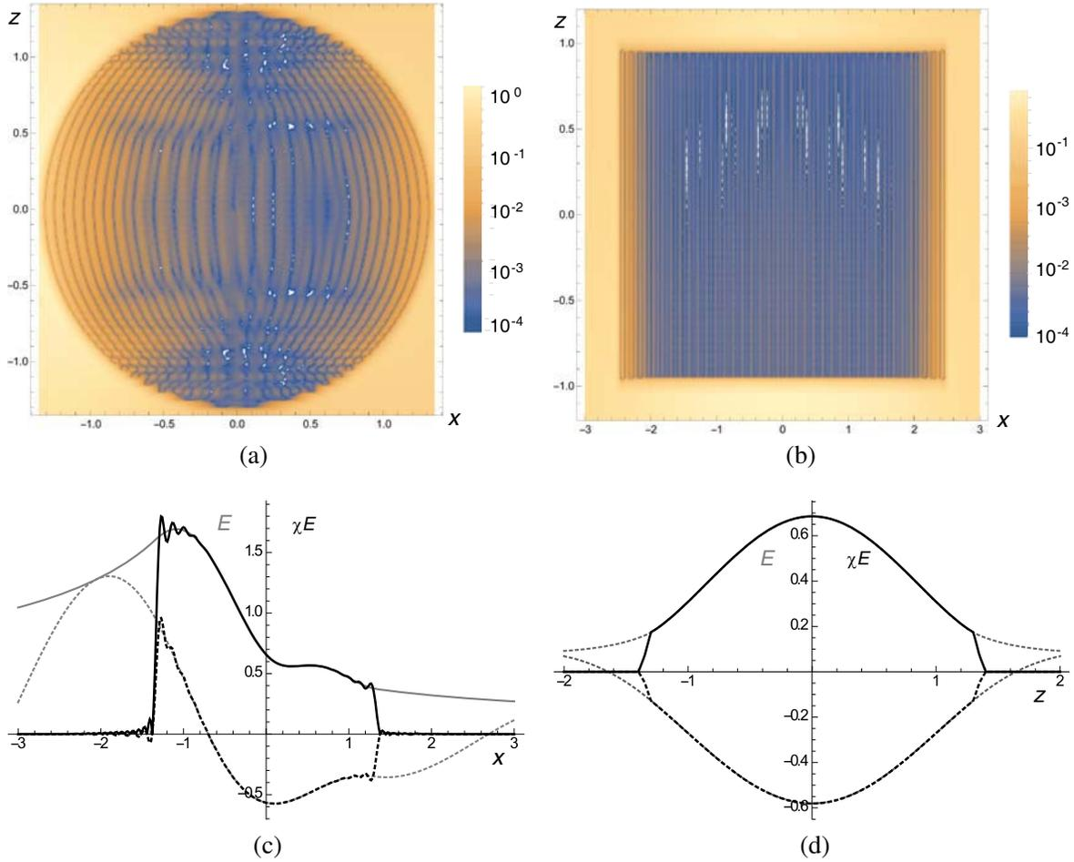
**Figure 7.** In (a) and (b) we plotted the absolute difference (error) between the electric field from the validation  $E$  and  $\chi E$  from our simulation results for the circle resp. the rectangle. At the scatterer these should coincide. In (c) we plotted the real (solid) and imaginary (dotted) part of  $E$  from validation (grey) and  $\chi E$  (black) from our simulation at  $z = -0.2$  for the circle. In (d) we did the same for a vertical cut along  $x = 0$  for the rectangle.
