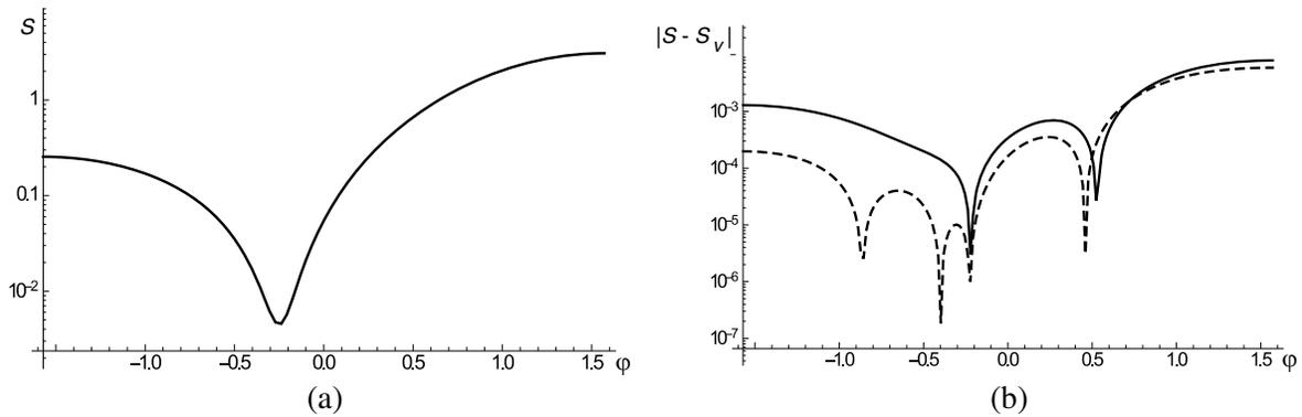
**Figure 8.** (a) The scattering intensity as calculated from the contrast current. (b) The absolute difference between the scattering intensity  $S$  and validation data  $S_V$ , the solid line is with the contrast current from the simulation, the dashed line is with the contrast current from the exact solution, represented by the same discretization as the simulation.
