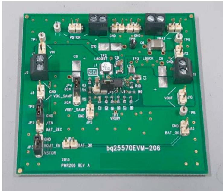
**Figure 10.** Fabricated BQ25570 power management circuit.
