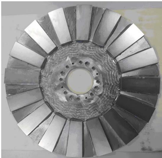
**Figure 7.** Axial flux machine rotor.
