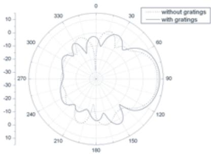
Figure 7. *E*-plane at 10 GHz.
