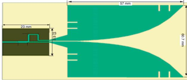
**Figure 1.** Geometry of the antenna.
