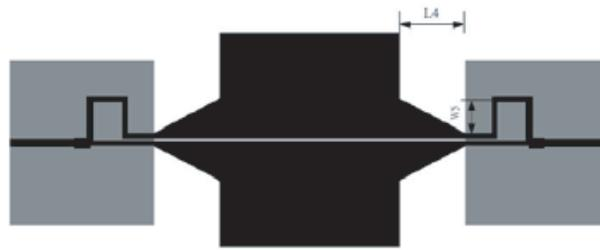
**Figure 2.** Conversion and connection of single plane and back to back between the microstrip and the slot line.
