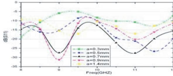
**Figure 3.**  $S_{11}$  about different slot width.
