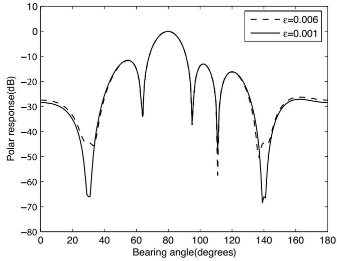
**Figure 3.** The beam pattern with different  $\epsilon$ .
