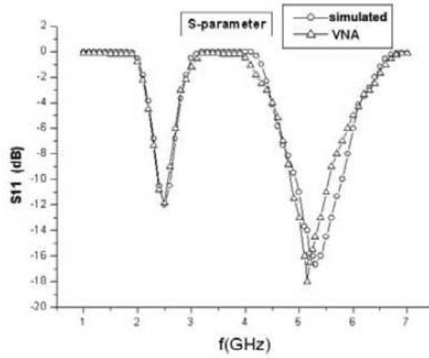
Figure 3. Simulated and measured  $S_{11}$ .
