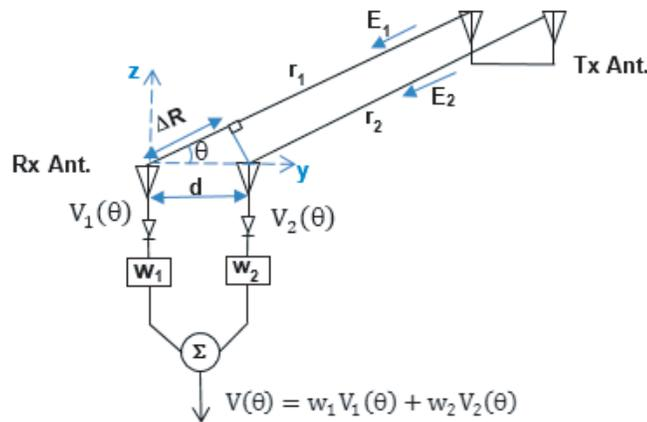
**Figure 1.**  $2 \times 2$  precoded MIMO smart antenna.
