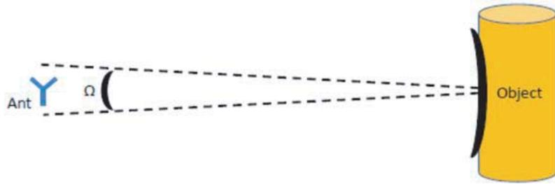
**Figure 1.** Antenna solid angle.
