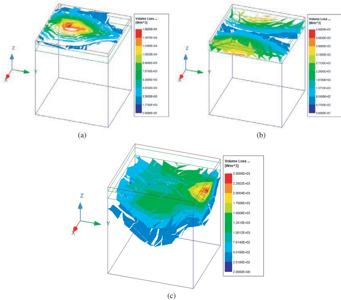
Figure 6. Simulated volume loss density for 1 V of input voltage at the antenna port, (a) skin, (b) fat, and (c) muscle.
