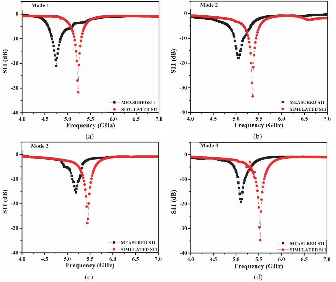
**Figure 4.** Simulated and measured  $S_{11}$  for different modes.
