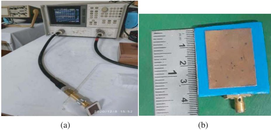
**Figure 18.** Measurement of return loss for the hook shaped aperture coupled circularly polarized antenna and proposed antenna prototype.
