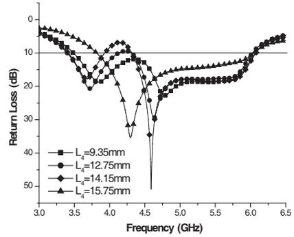
**Figure 6.** Effect of variation of slot length  $L_4$  on return loss.
