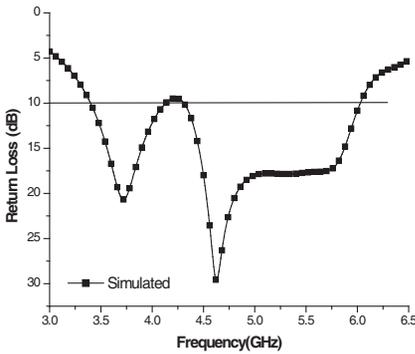
**Figure 3.** Simulated return-loss of proposed antenna.
