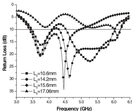
Figure 7. Effect of variation of slot length  $L_5$  on return loss.
