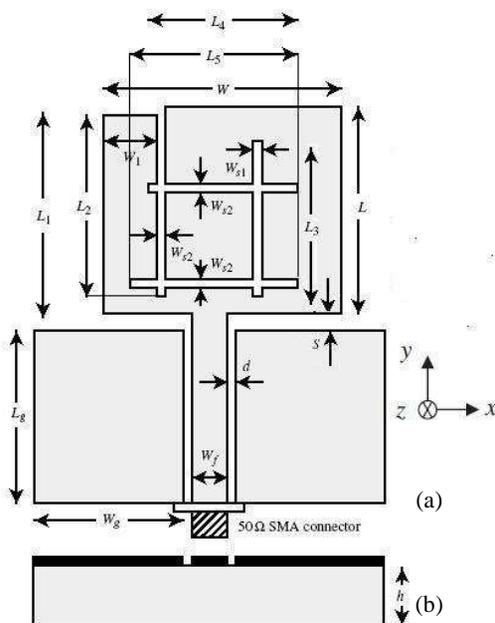
**Figure 1.** Geometry of the proposed antenna. (a) Top view, (b) front view.
