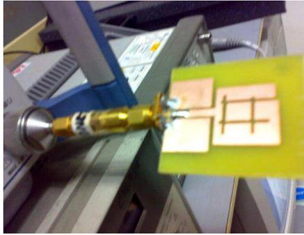
**Figure 2.** Fabricated antennas with proposed design.
