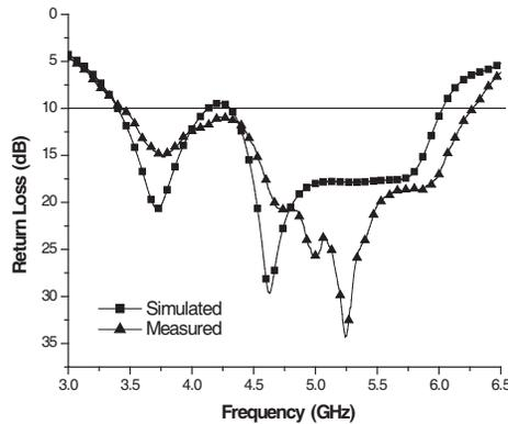
**Figure 11.** Simulated and measured return-losses of proposed antenna.
