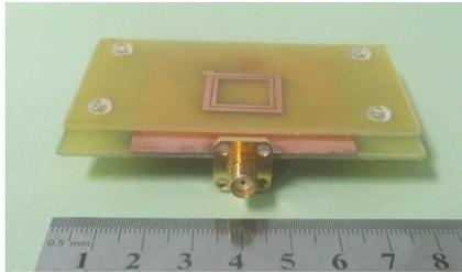
**Figure 9.** Photograph of proposed antenna.
