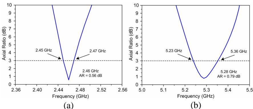
Figure 6. AR Spectrum. (a) 2.46 GHz, (b) 5.28 GHz.
