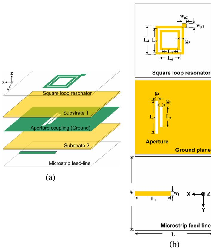
**Figure 3.** Configuration of proposed antenna. (a) Structure, (b) configuration with the dimensions.
