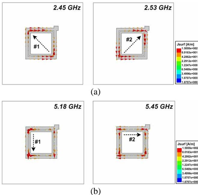
Figure 5. Vector current distributions. (a) 2.46 GHz, (b) 5.28 GHz.
