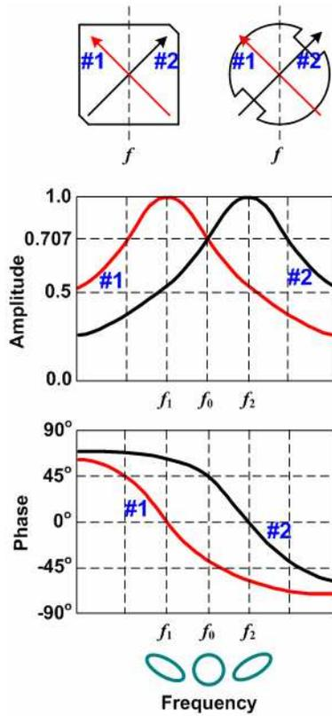
**Figure 2.** Orthogonal mode of single-point feed square patch.
