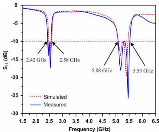
Figure 4. Results of return loss spectrum.
