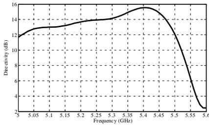
**Figure 10.** Directivity evolution versus frequency.
