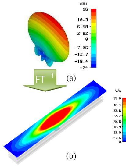
**Figure 3.** (a) 3D radiation pattern of a rectangular sectoral M-EBG antenna, (b) elliptical aperture.
