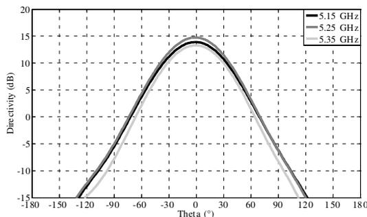
**Figure 28.** Radiation patterns in the horizontal plane.
