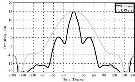
**Figure 8.** Radiation patterns at 5.29 GHz.
