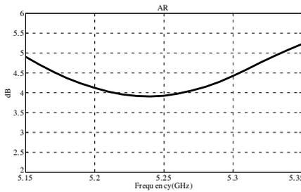
**Figure 22.** Axial Ratio versus frequency.
