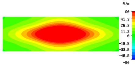
**Figure 5.** Field distribution inside the sectoral M-EBG antenna.
