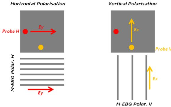
**Figure 13.** A patch antenna with two feed probes.
