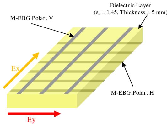
**Figure 12.** Geometry of the upper M-EBG structure.
