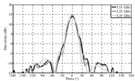
**Figure 27.** Radiation patterns in the vertical plane.
