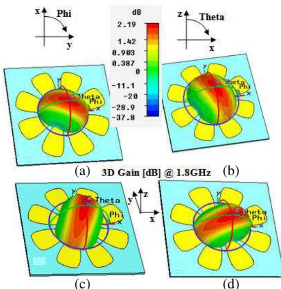
**Figure 5.** Radiation pattern calculated by means of full-wave simulations performed with CST Microwave Studio. (a)–(d) Three-dimensional gains obtained for configurations 1–4 of the antenna illustrated in Fig. 2(b).
