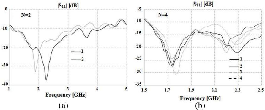
**Figure 8.** Measurements of the reflection coefficient for the antennas illustrated in Fig. 5. (a) Experimental data obtained for the two possible configurations of the antenna of Fig. 5(a). (b) Experimental data obtained for the four possible configurations of the antenna of Fig. 5(b).
