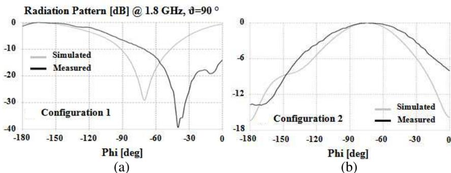
**Figure 9.** Experimental results obtained for the radiation pattern of the antenna illustrated in Fig. 5(a) corresponding to the application of the proposed approach for the case  $N = 2$ . Radiation patterns measured for configuration 1 (i.e., vertical bowtie activated) (a) and configuration 2 (b) (i.e., horizontal bowtie activated).
