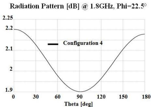
**Figure 6.** Full-wave simulations results obtained for the radiation pattern corresponding to configuration 4 of the antenna illustrated in Fig. 2(b). The value set for  $\Phi$  identifies the  $H$ -plane of the proposed antenna when it is in configuration 4.
