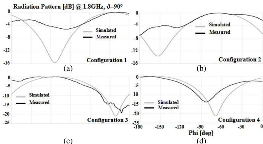
**Figure 10.** Experimental results obtained for the radiation pattern of the antenna illustrated in Fig. 5(b) corresponding to the application of the proposed approach for the case  $N = 4$ . (a)–(d) Radiation patterns measured for configurations 1–4.
