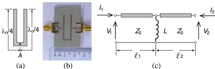
**Figure 1.** (a) Hair-pin resonator with a via at the centre.  $\lambda_0$  is the wavelength of the fundamental resonant frequency,  $f_0$  of the resonator without a via. (b) Photograph of the resonator with weak coupling. (c) Equivalent circuit of a hair-pin resonator with a via.  $\ell_1$  and  $\ell_2$  are the lengths of the two arms measured from the grounding via.
