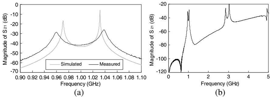
**Figure 2.** (a) Simulated and measured variation of the magnitude of  $S_{21}$  using the frequency for equal arm length hair-pin resonator with a via. The arm length is 29 mm. The centre frequency,  $f_C$  is 1.0 GHz. (b) Simulation broadband response of  $S_{21}$ .
