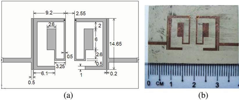
**Figure 8.** (a) Layout of the 4-pole bandpass filter designed using the proposed compact resonator. (b) Photograph of the fabricated 4-pole bandpass filter.
