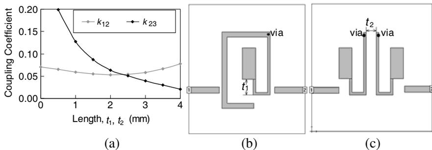
**Figure 7.** (a) Design curve for the coupling coefficients,  $k_{12}$  and  $k_{23}$ . The layout of the resonators to obtain the design curve for (b) the coupling coefficient value of  $k_{12}$  varies with length  $t_1$  and (c) the coupling coefficient value of  $k_{23}$  varies with length  $t_2$ .
