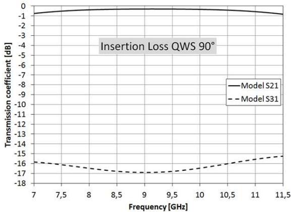
**Figure 5.** Insertion loss of  $QWS_{90^\circ}$ .
