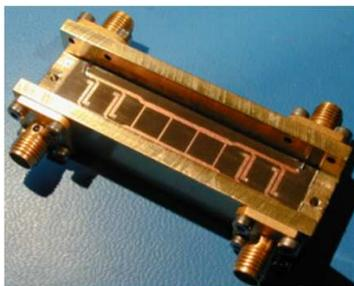
Figure 8. Branch-line coupler prototype.
