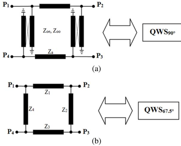
**Figure 3.** Correspondence between the branch-line couplers with arbitrary power division and the two QWSs of interest: QWS<sub>67.5°</sub> and QWS<sub>90°</sub>.
