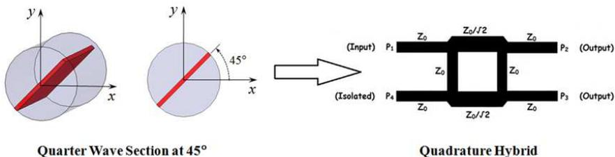
**Figure 1.** A planar quadrature hybrid is equivalent to a waveguide polarizer rotated by  $45^\circ$  setting a correspondence between the  $x$  and  $y$  polarized modes and port 1 and 4 of the hybrid.
