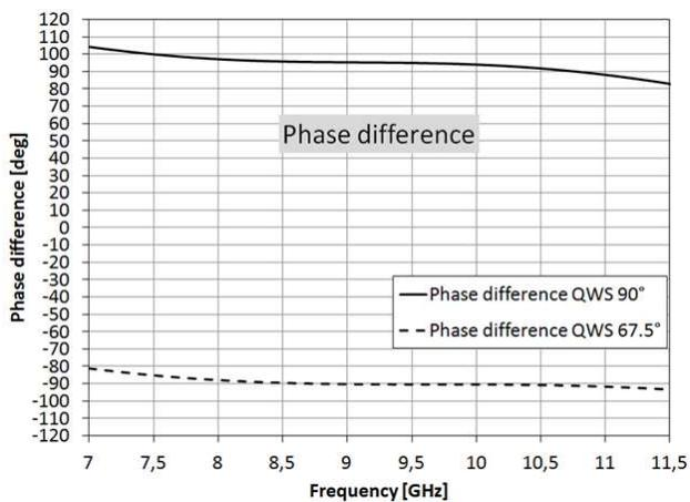
Figure 6. Phase difference of  $QWS_{67.5^\circ}$  and  $QWS_{90^\circ}$ .
