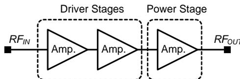
**Figure 1.** General power amplifier structure.
