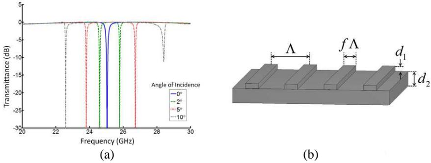
**Figure 1.** Baseline GMRF in HDPE ( $\epsilon_r = 2.35$ ) which has  $\Lambda = 9.19$  mm,  $f = 0.36$ ,  $d_1 = 1.19$  mm, and  $d_2 = 3.35$  mm. (a) Simulated transmission at several angles of incidence. (b) Geometry of baseline design.
