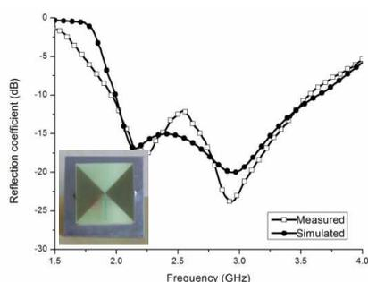
**Figure 6.** Measured and simulated reflection coefficient of the antenna.
