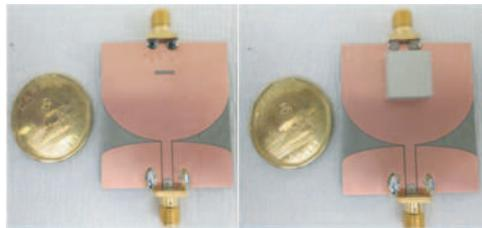
**Figure 4.** The photo of fabricated antenna prototype.
