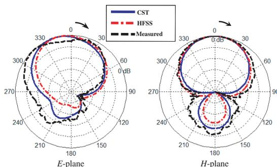
**Figure 7.** Radiation patterns for narrow-band antenna at 5.8 GHz.
