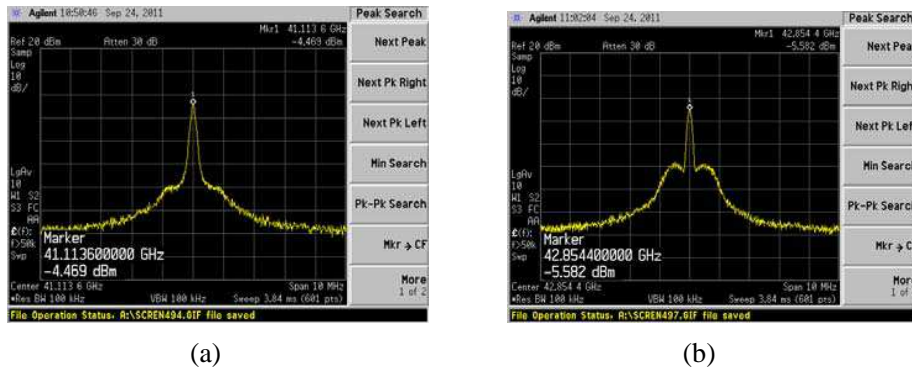
Figure 13. Measured output spectrum: (a) 41.11 GHz and (b) 42.85 GHz.
