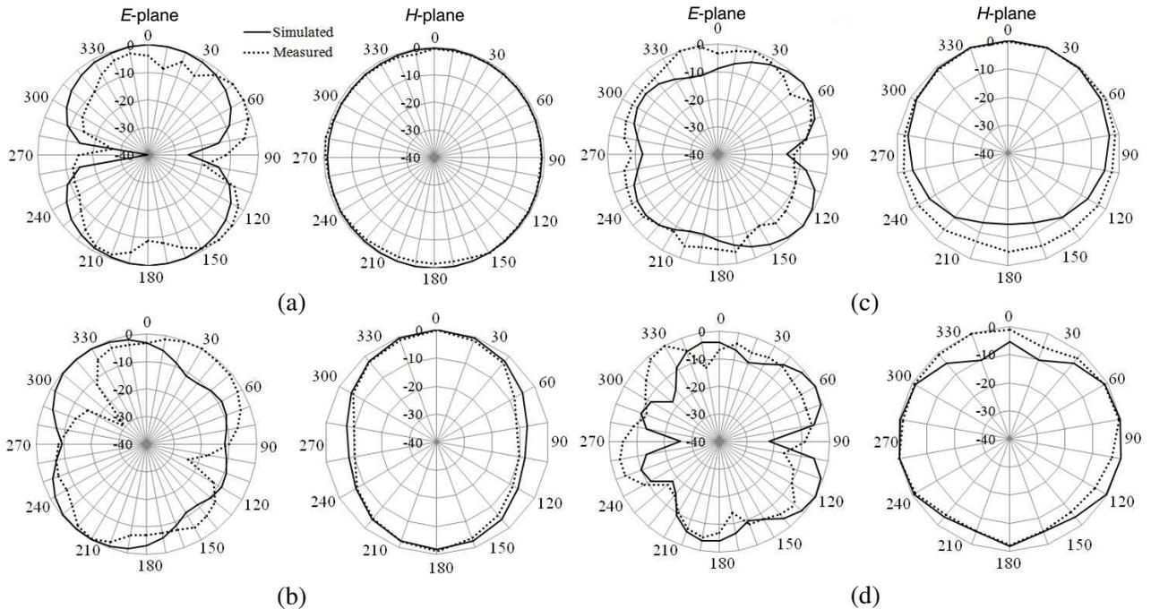
**Figure 8.** *E*-plane and *H*-plane radiation patterns of proposed compact planar monopole UWB antenna with quadruple band-notched characteristics at various frequencies of (a) 3 GHz, (b) 5.8 GHz, (c) 8 GHz, and (d) 10 GHz.
