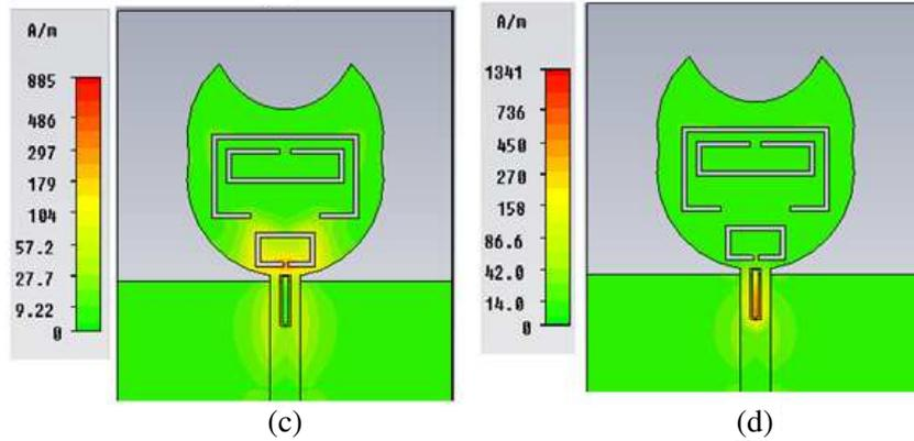
**Figure 7.** Simulated magnitude of current distribution at (a) 2.56 GHz, (b) 3.7 GHz, (c) 5.8 GHz, and (d) 8 GHz of proposed compact planar monopole UWB antenna with quadruple band-notched characteristics.
