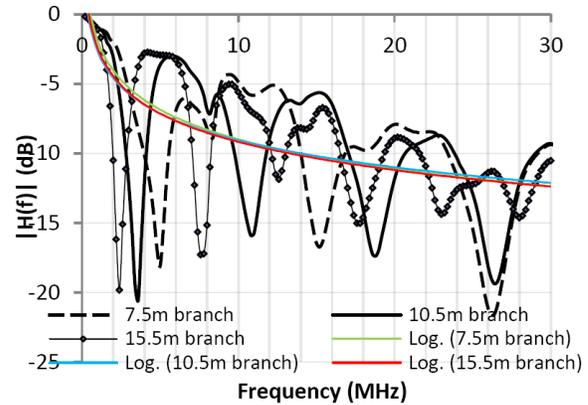
Figure 7. Measurement results for variation in branch length of the same network.
