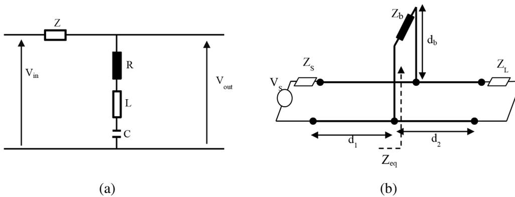
**Figure 8.** (a) The series resonant circuit. (b) The T-node topology connected to source and load.
