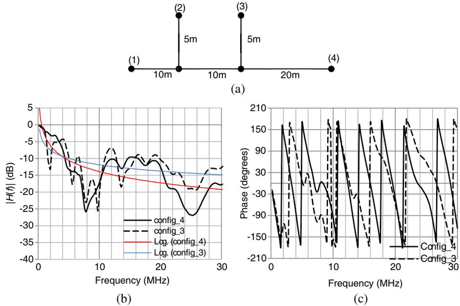
**Figure 4.** (a) Illustration of a two T-node topology. (b) The transfer function for two configurations of the two T-node topology. (c) The phase response for two configurations of the two T-node topology.
