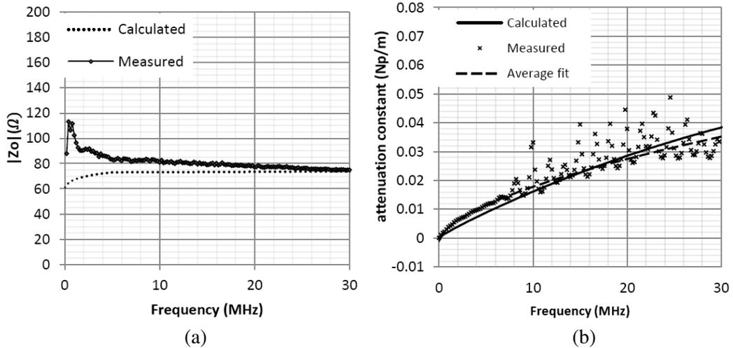
**Figure 1.** (a) The characteristic impedance for the  $2.5 \text{ mm}^2$  transmission line. (b) The measured and calculated attenuation coefficient for the  $2.5 \text{ mm}^2$  cable.
