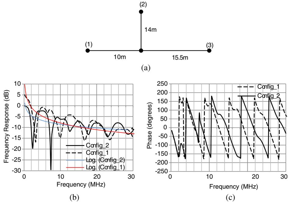
**Figure 3.** (a) The T node topology. (b) The transfer function for different configurations of the T node topology. (c) The phase response for different configurations of the T node topology.
