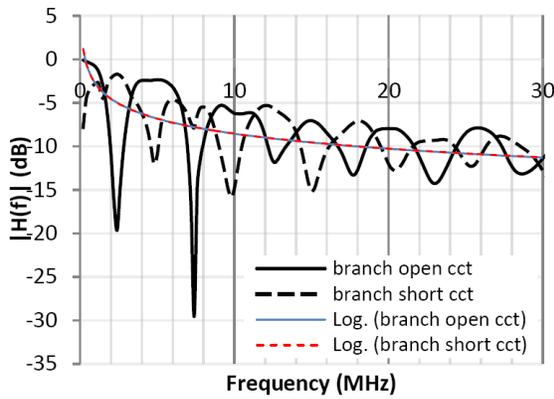
Figure 6. The transfer function for a T-node with branch end short circuited and open circuited.
