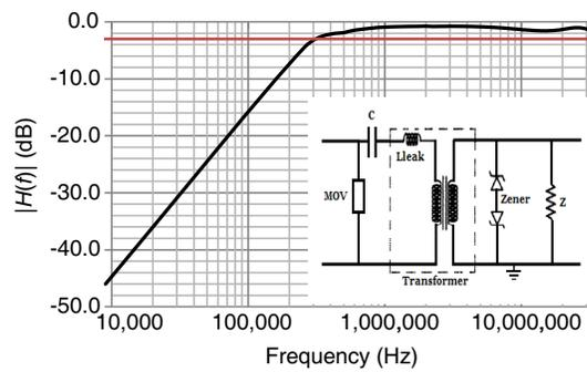
**Figure 2.** The coupler design and transfer function.
