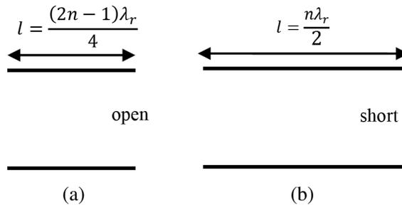
**Figure 9.** Types of transmission line series resonant circuits with length (a) a quarter wavelength and (b) a half wavelength.
