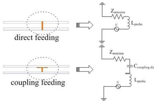
**Figure 3.** Equivalent circuit of the coupling feed in the proposed dual-band dual-sense CP microstrip antenna.
