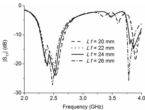
**Figure 8.** Simulated  $|S_{11}|$  with different slot length  $L_1$  for the proposed dual-band dual-sense CP microstrip antenna.
