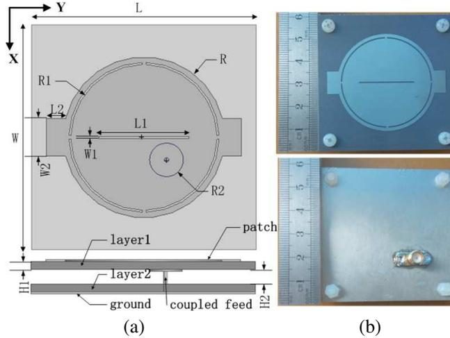
**Figure 1.** Geometry and photograph of the proposed dual-band dual-sense CP micro-strip antenna. (a) Geometry. (b) Photograph.
