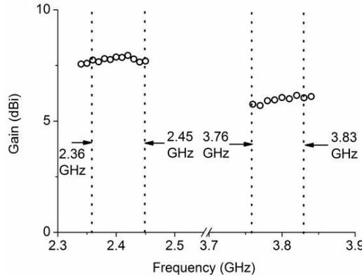
**Figure 7.** The measured peak gains of the proposed dual-band dual-sense CP micro-strip antenna.
