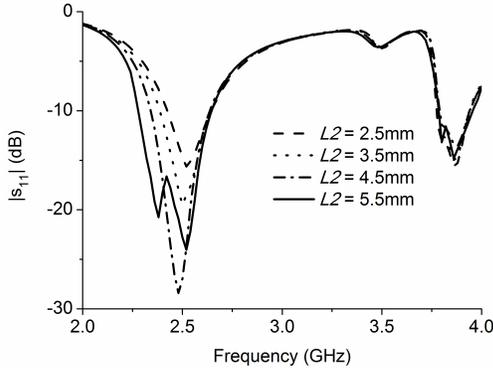
**Figure 10.** Simulated  $|S_{11}|$  with different stub length  $L_2$  for the proposed dual-band dual-sense CP microstrip antenna.
