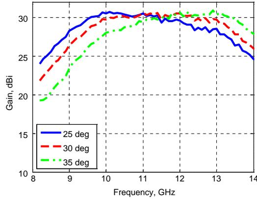
**Figure 9.** Measured gain of the  $0.3\lambda$  reflectarray with scan angles of  $25^\circ$ ,  $30^\circ$  and  $35^\circ$ .
