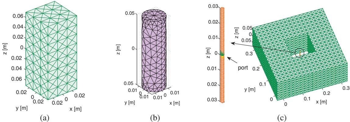
**Figure 1.** Reconfigurable PAA: (a) 3-D triangular tessellation of a cuboidal brick’s surface and (b) tetrahedral mesh of a cylindrical plasma discharge; (c) LEGO model showing  $N_D = 32$  EM bricks in the case where all the plasma discharges are energized and (inset) a close-up of the 3-D triangular-faceted model of the PEC dipole antenna.
