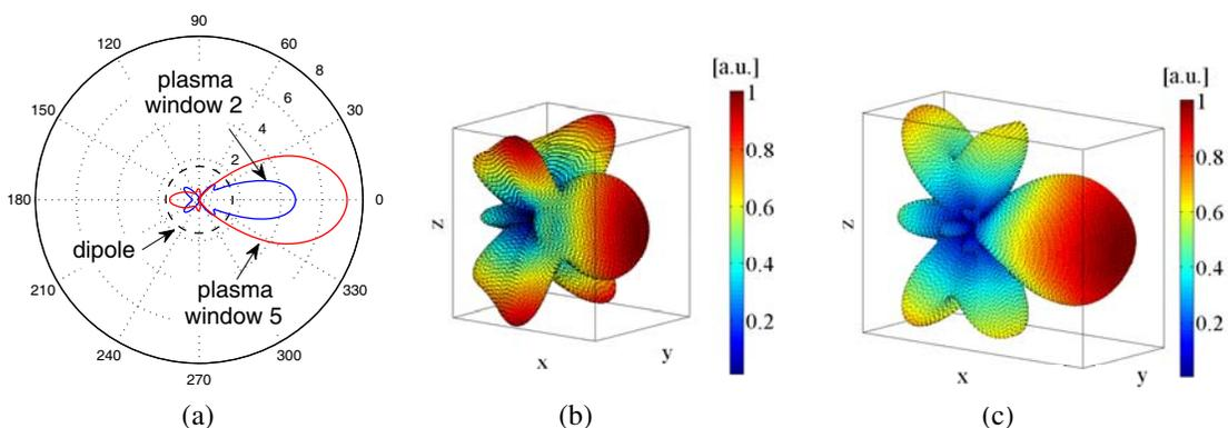
**Figure 5.** Reconfigurable PAA: (a) Antenna gain  $g(90^\circ, \phi)$  for the configurations shown in Figs. 2(c) and 2(d) and  $B_0 = 0$ ,  $n_e = 10^{18} \text{ m}^{-3}$ ; (b), (c) 3-D radiation pattern  $|\mathbf{E}^s(\theta, \phi)|/|\mathbf{E}^s(\theta, \phi)|_{\max}$  for the configurations of Figs. 2(c) and 2(d), respectively, and  $B_0 = 0$ ,  $n_e = 10^{18} \text{ m}^{-3}$ .
