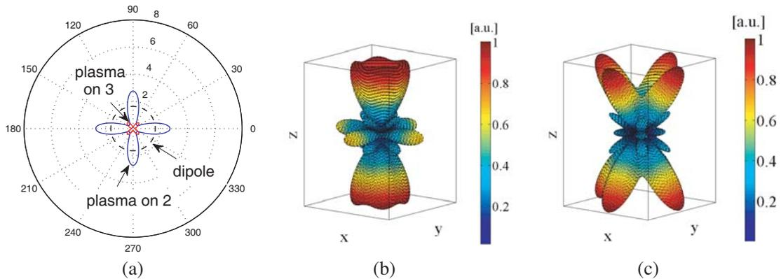
**Figure 4.** Reconfigurable PAA: (a) Antenna gain  $g(90^\circ, \phi)$  for the configurations shown in Figs. 2(a) and 2(b) and  $B_0 = 0$ ,  $n_e = 10^{18} \text{ m}^{-3}$ ; (b), (c) 3-D radiation pattern  $|\mathbf{E}^s(\theta, \phi)|/|\mathbf{E}^s(\theta, \phi)|_{\max}$  for the configurations of Figs. 2(a) and 2(b), respectively, and  $B_0 = 0$ ,  $n_e = 10^{18} \text{ m}^{-3}$ .
