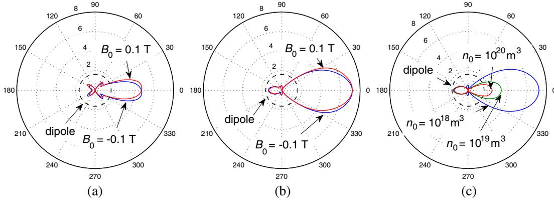
**Figure 6.** Reconfigurable PAA: (a), (b) Effect of a static magnetic field on the antenna gain  $g(90^\circ, \phi)$  for the configurations shown in Figs. 2(c) and 2(d), respectively, and  $n_e = 10^{18} \text{ m}^{-3}$ ; (c) Effect of the plasma density on the antenna gain  $g(90^\circ, \phi)$  for the configuration of Fig. 2(d) and  $B_0 = 0$ .
