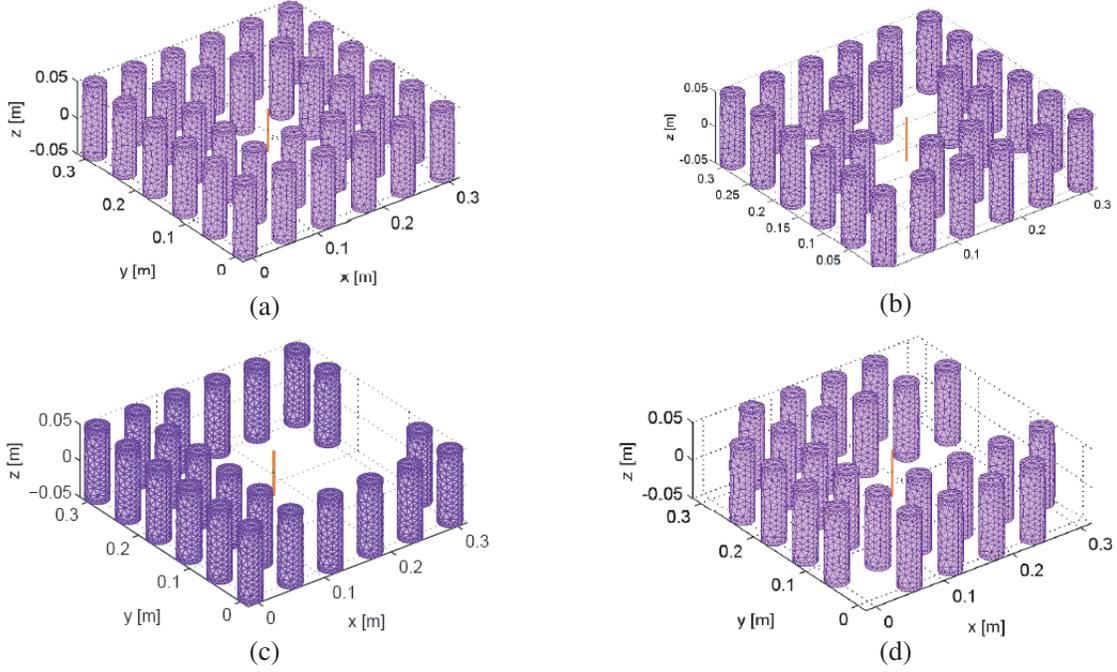
**Figure 2.** Reconfigurable PAA, LEGO models: (a) Configuration “plasma on 2” composed of  $N_D = 32$  energized plasma discharges; (b) Configuration “plasma on 3” comprised of  $N_D = 28$  energized plasma discharges; (c) Configuration “plasma window 2” composed of  $N_D = 22$  energized plasma discharges; (d) Configuration “plasma window 5” composed of  $N_D = 24$  energized plasma discharges. (Remark: inactive discharges, when present, are not shown.)
