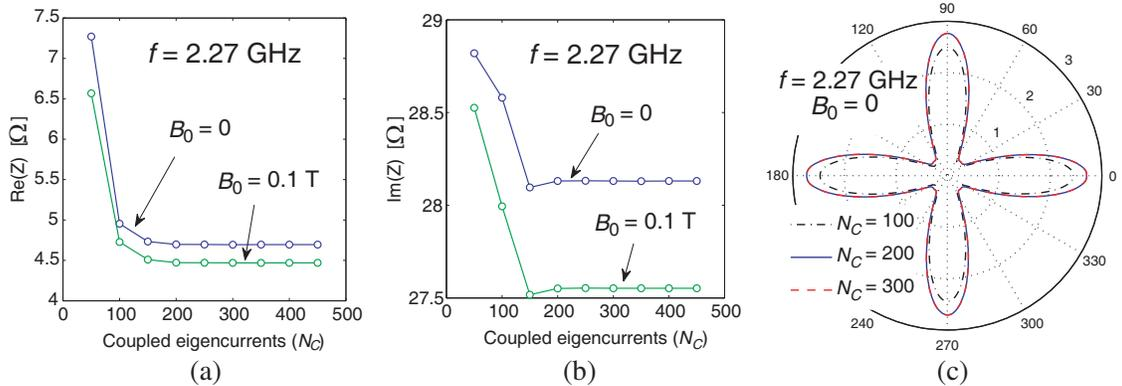
**Figure 3.** Reconfigurable PAA: Convergence of solution computed with LEGO and EEM as a function of the number of coupled eigencurrents  $N_C$  for the configuration “plasma on 2” shown in Fig. 2(a); (a) Real part of antenna impedance; (b) Imaginary part of antenna impedance; (c) Antenna gain  $g(90^\circ, \phi)$ .
