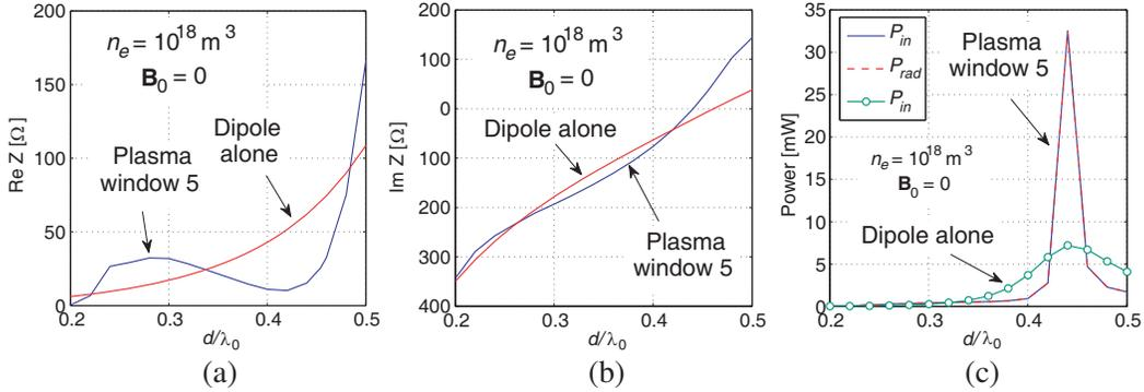
**Figure 7.** Reconfigurable PAA: Impedance and powers as a function of the electric length of the dipole for the configuration “plasma window 5” shown in Fig. 2(d); (a) Real part; (b) Imaginary part, and (c) input and radiated powers when the PAA is energized with  $V_G = 1$  V in the delta-gap model of the feed.
