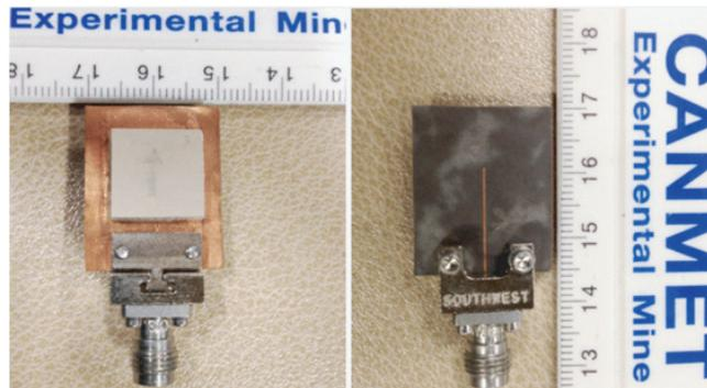
**Figure 14.** Photograph of the proposed antenna.
