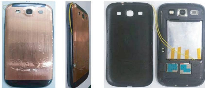
**Figure 8.** Prototype antenna with a mobile phone.
