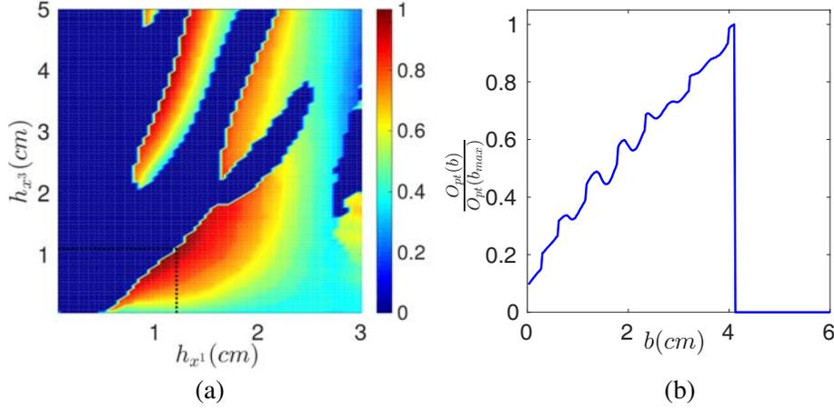
**Figure 5.** Evolution of the normalized target function  $O_{pt}$ . Excitation is done with the fundamental TE mode. (a) Parametric study by varying the two dimensions of the rectangular tip. (b) Parametric study by varying the depth of the elliptical tip.
