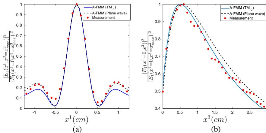
**Figure 11.** Measurement and simulation results of the normalized electric intensity at 30 GHz for the TM polarization ( $h_{x^1} = 1$  cm and  $h_{x^3} = 0.75$  cm).  $h = 3\lambda$ . (a) Cross section at the maximum of the photonic jet. (b) Longitudinal section at  $x^1 = 0$  cm.
