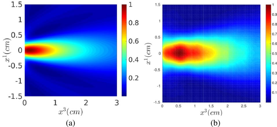
**Figure 8.** (a) Numerical results obtained by A-FMM for the rectangular tip chosen for the experimental validation  $h_{x^1} = 1$  cm and  $h_{x^3} = 0.75$  cm when  $h = 3\lambda$  with  $\lambda = 1$  cm excited by the fundamental mode ( $TE_1$ ). (b) Measurement of the normalized intensity of electric field, obtained with the free space excitation.
