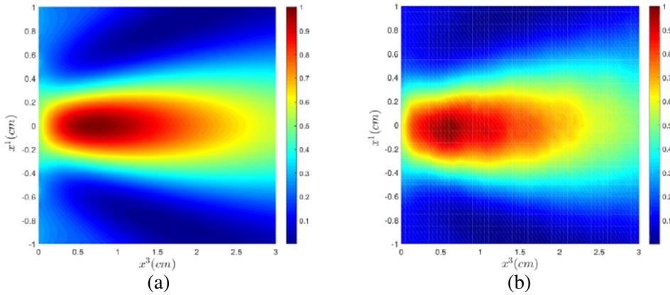
**Figure 10.** (a) Numerical results obtained by FMM for the rectangular tip ( $h_{x^1} = 1$  cm and  $h_{x^3} = 0.75$  cm) excited by the fundamental mode ( $TM_0$ ). (b) Measurement of the normalized intensity of electric field at 30 GHz.  $h = 3\lambda$  with  $\lambda = 1$  cm.
