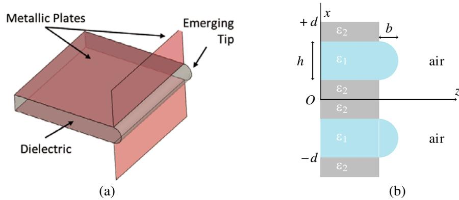
**Figure 1.** (a) Parallel plate waveguide under study (3D vision). (b) Periodical structure obtained using FMM (Side view of 2 elementary cells of the gratings).
