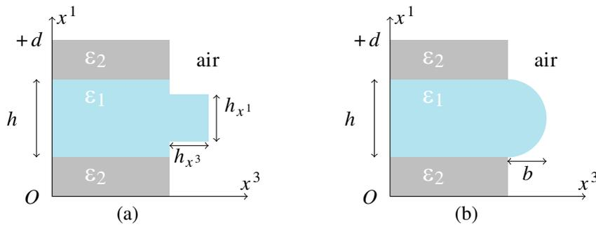
**Figure 4.** A schematic drawing of a parallel plate waveguide ended with: (a) a rectangular tip or (b) an elliptical tip.
