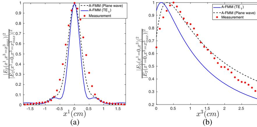
**Figure 9.** Comparisons for the normalized electric intensity between measurement and simulations. (a) Cross section at the maximum of the photonic jet. (b) Longitudinal section of the photonic jet at  $x^1 = 0$  cm.
