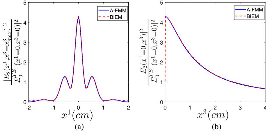
**Figure 3.** Comparisons between a-FMM method and integral approach results for the elliptical tip ( $b = 4\lambda$ ,  $h = 3\lambda$ ). *TE* polarization at 30 GHz ( $\lambda = 1$  cm).  $E_0^{TE1}$  is the electric field of the fundamental mode in the waveguide and  $E_2$  the  $x^2$ -component of the electric field in the air. (a) Cross section at the maximum of the photonic jet ( $x^3 = x^3_{\max}$ ). (b) Longitudinal section of the photonic jet at  $x^1 = 0$  cm.
