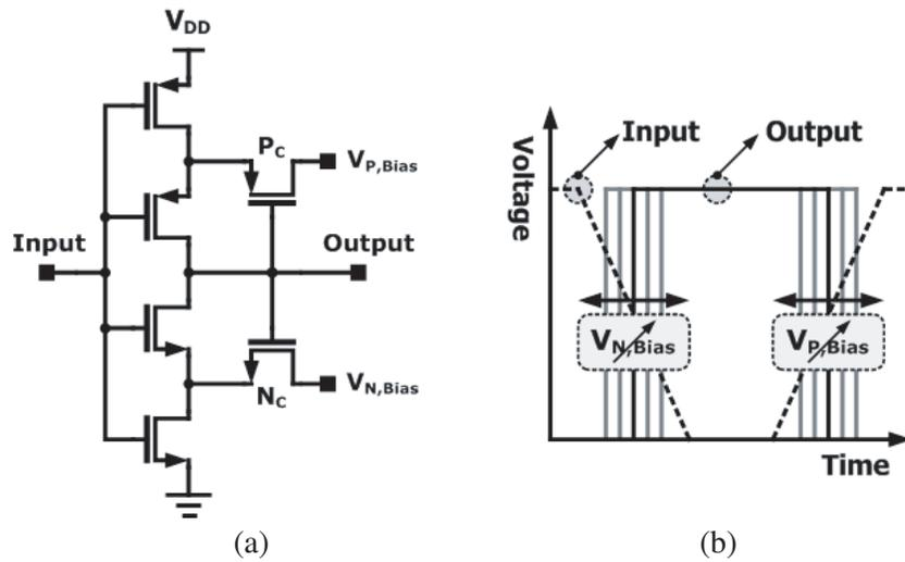
Figure 11. Proposed Schmitt trigger.
