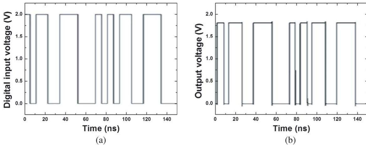
**Figure 12.** Simulation results: (a) digital input and (b) output voltage waveform of the Schmitt trigger.
