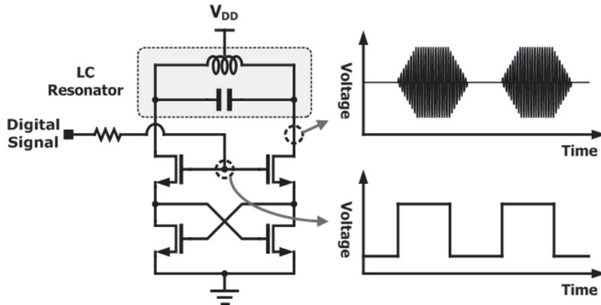
**Figure 7.** Proposed voltage-controlled oscillator.
