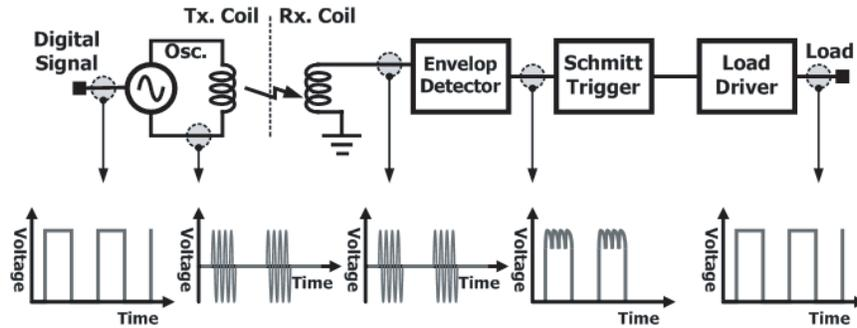
**Figure 6.** Block diagram of the proposed transceiver.
