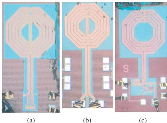
**Figure 13.** Chip photographs: (a) transmitter, (b) coil of the receiver, and (c) receiver.
