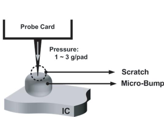
**Figure 3.** Conceptual diagram of on-wafer probing on a micro-bump.
