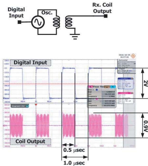
Figure 15. Digital input and measured output voltage waveform at the receiver coil.
