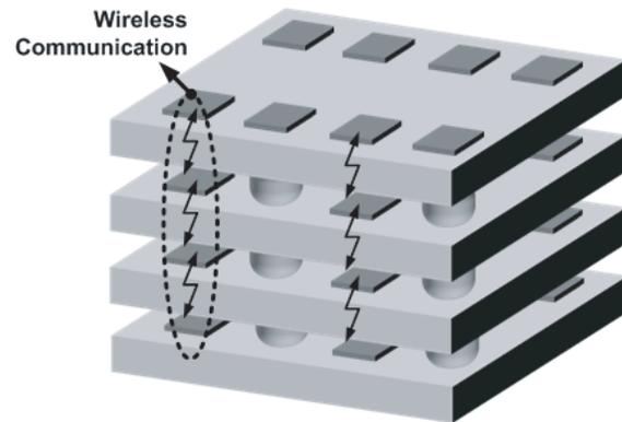
**Figure 4.** Conceptual diagram of wireless chip-to-chip communication.
