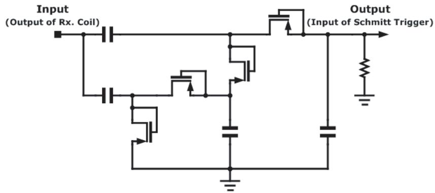
Figure 9. Designed envelope detector.
