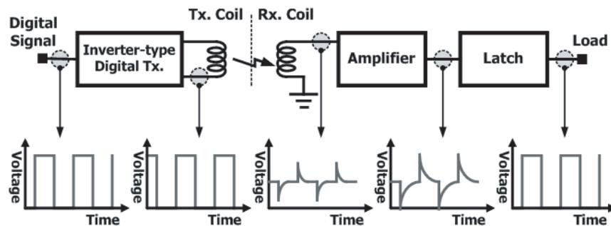
**Figure 5.** Block diagram of a pulse-type transceiver for WCC technology [8].
