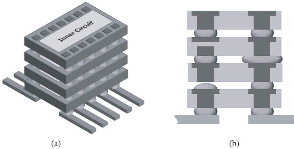
**Figure 2.** TSV technology: (a) conceptual diagram and (b) general case of failures.
