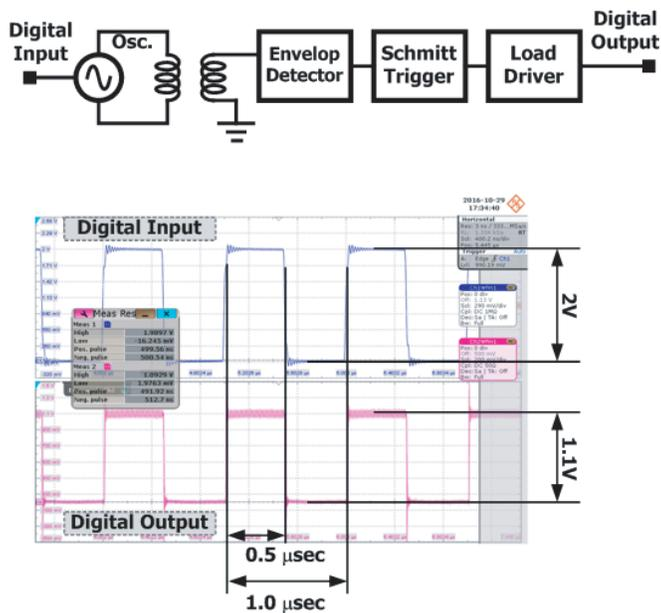
Figure 17. Digital input and measured output voltage waveform of the proposed transceiver.
