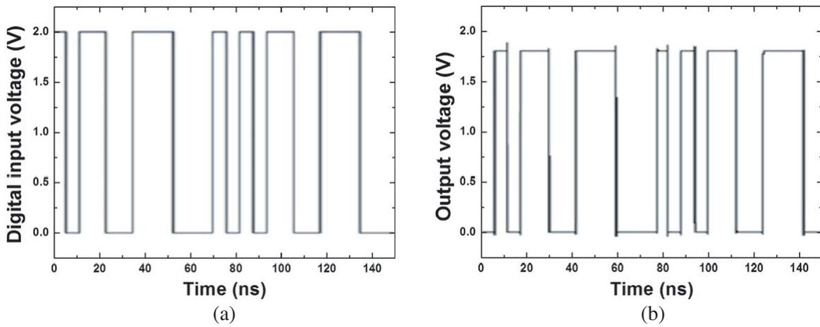
Figure 10. Simulation results: (a) digital input and (b) output voltage waveform of the envelope detector.
