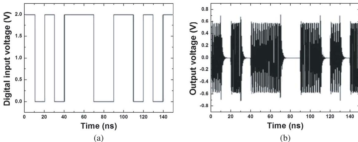
**Figure 8.** Simulation results: (a) digital input and (b) output voltage waveform of oscillator.
