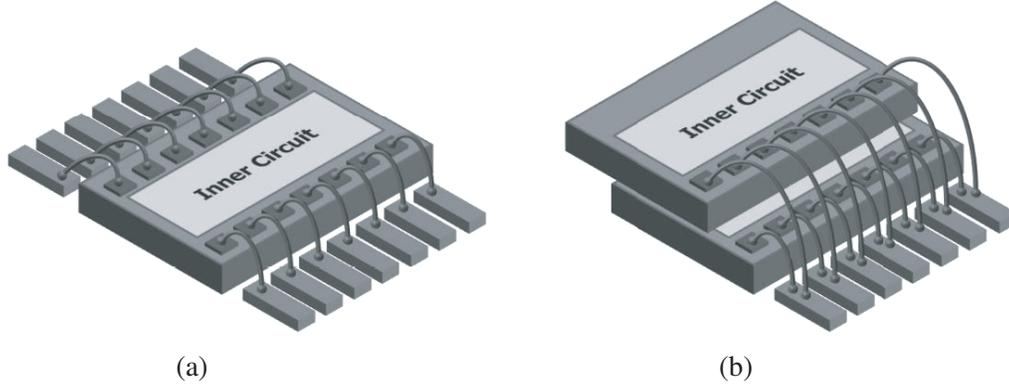
**Figure 1.** Typical semiconductor technology: (a) 2D semiconductor and (b) MCP technologies.
