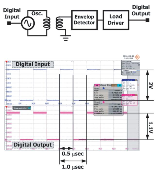
Figure 16. Digital input and measured output voltage waveform with the envelope detector of the transmitter.
