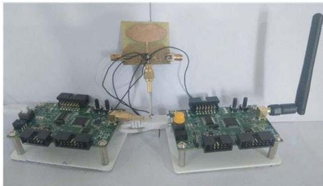
**Figure 20.** Connecting fabricated antenna to CDAC Cmote.
