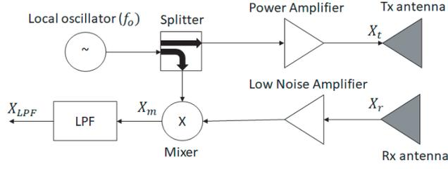
**Figure 2.** Block Diagram of 10 GHz CW radar system.
