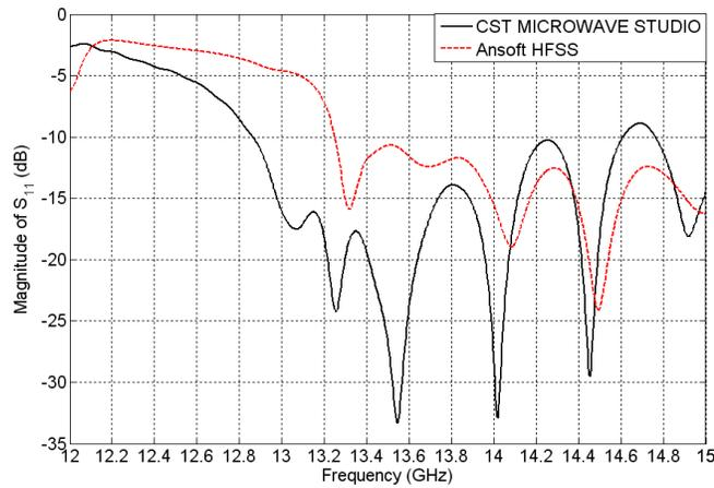
**Figure 3.** Magnitude of  $S_{11}$  for proposed antenna in dB.
