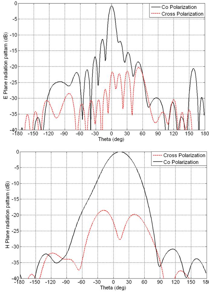
**Figure 6.** Radiation patterns simulated in  $f = 13.7$  GHz, top is  $\varphi = 90^\circ$  cut and bottom is  $\varphi = 0^\circ$  cut.
