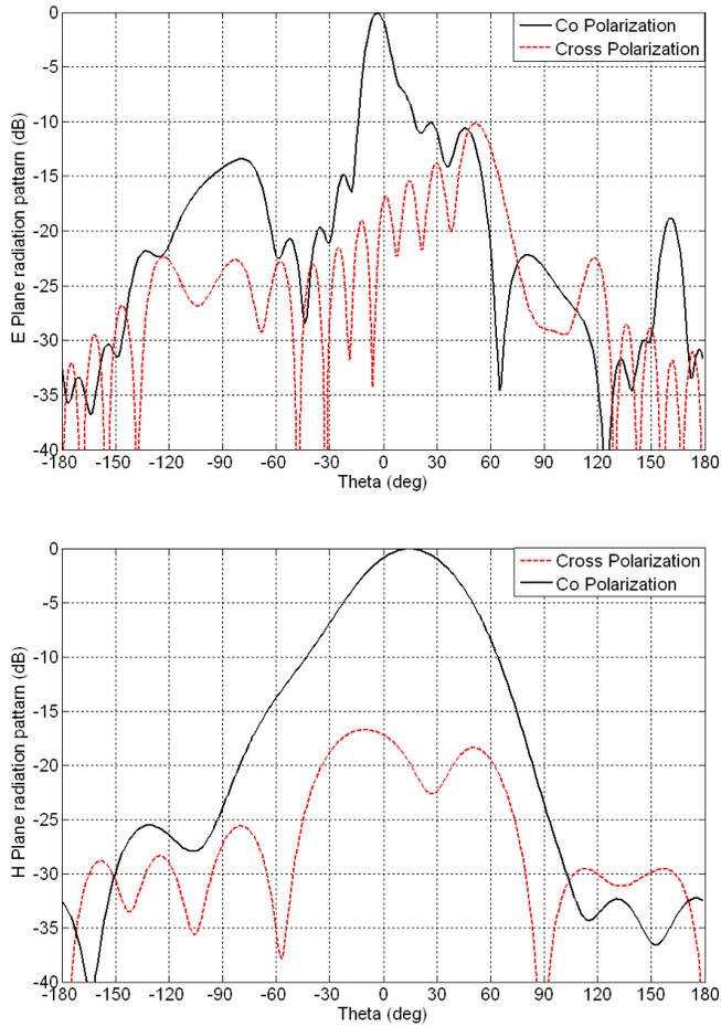
**Figure 5.** Radiation patterns simulated in  $f = 13.4\text{GHz}$ , top is  $\varphi = 90^\circ$  cut and bottom is  $\varphi = 0^\circ$  cut.
