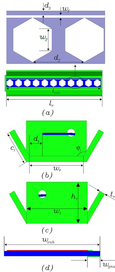
**Figure 1.** Geometrical parameters of antenna with band notch characteristics.
