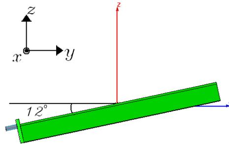
**Figure 4.** The deviation of antenna from Y-axis.
