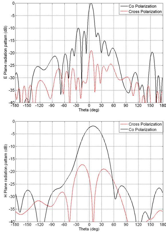
**Figure 7.** Radiation patterns simulated in  $f = 14.0$  GHz, top is  $\varphi = 90^\circ$  cut and bottom is  $\varphi = 0^\circ$  cut.
