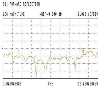
**Figure 4.** Measured return loss of the  $2 \times 2$  quasi-Yagi array fed by novel orthogonal T junction.
