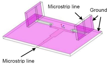
**Figure 2.** Configuration of novel orthogonal T junction.
