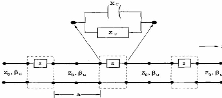
Figure 2. Equivalent circuit of periodic circuit representing PBG structure.
