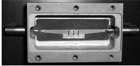
**Figure 3.** Fabricated broadband bandpass filter.
