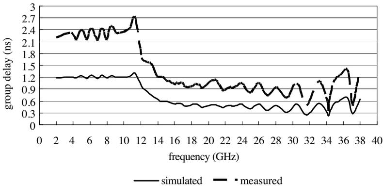
**Figure 5.** Measured and simulated  $S'_{21}$  group delay (at normal temperature).
