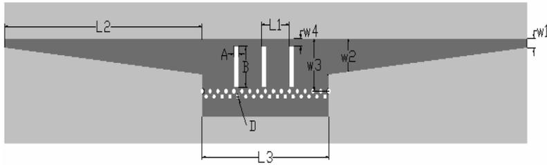
Figure 1. Circuit of broadband bandpass filter.
