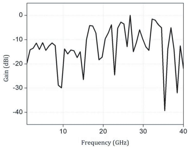
**Figure 5.** Gain of the textile antenna.
