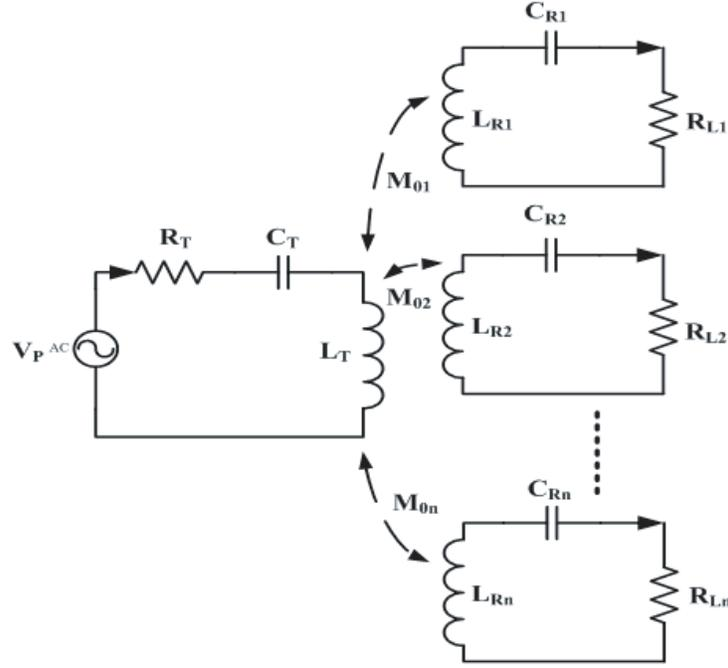
**Figure 1.** Circuit equivalent model of multi-receiver WPT system.
