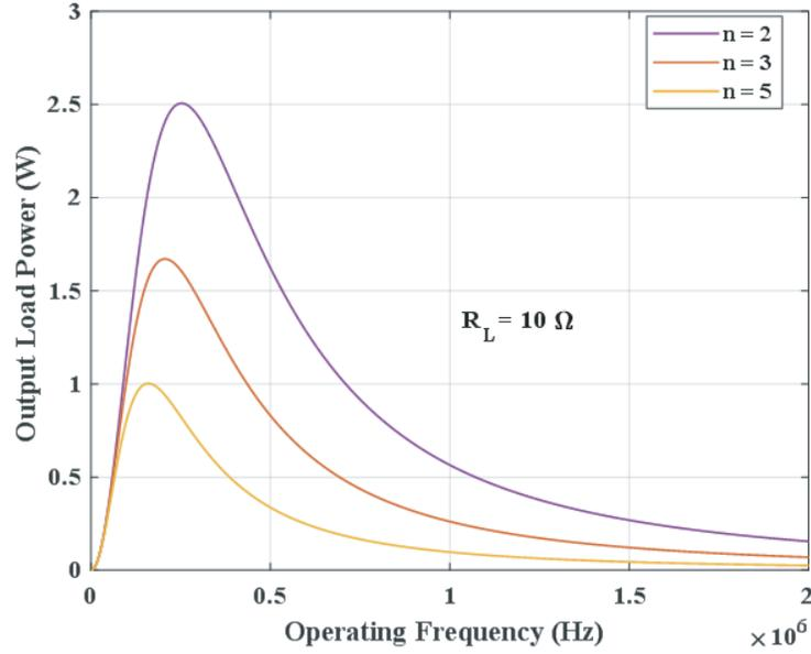
**Figure 3.** Frequency characteristics of output load power.
