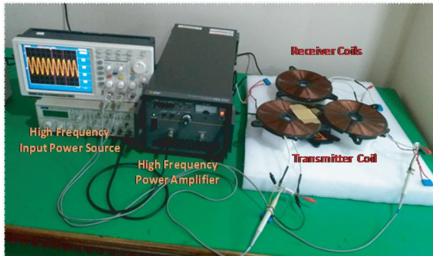
**Figure 2.** Experimental set up for three-Load WPT system.
