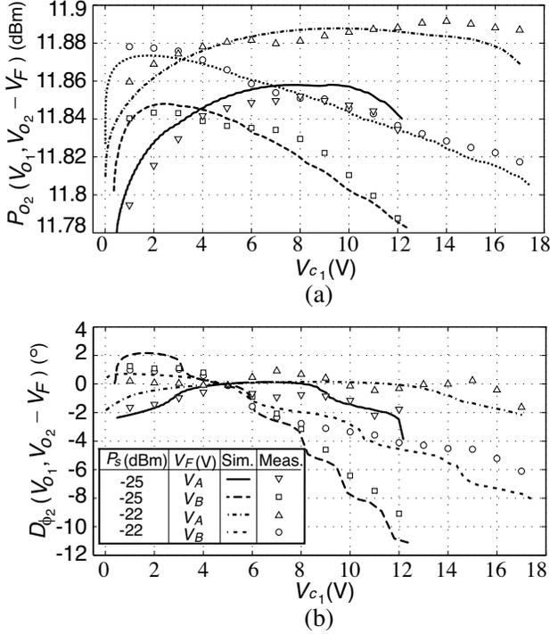
**Figure 3.** Variation of the output power  $P_{O_2}$  and the phase shift  $\Delta\phi_2$  of  $ILO_2$ , when its control voltage is kept at a fixed point  $V_{c_2} = V_F$ , as a function of the control voltage of  $ILO_1$  ( $V_{c_1}$ ). The measured values are shown together with the simulation results.
