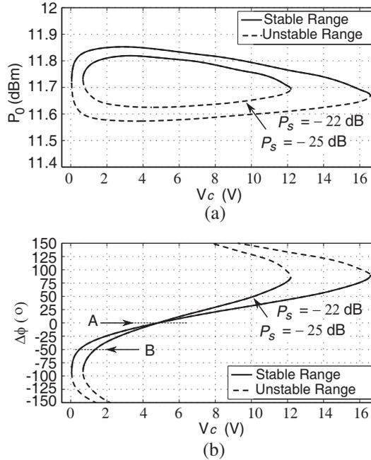
**Figure 2.** Synchronised operation loci as a function of the control voltage for: (a) The output power and (b) The phase shift, simulated for different synchronisation power levels. The stable regions of operation are also indicated.
