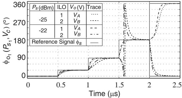
**Figure 4.** Phase transients of the output signals of the circuits  $\phi_{o_i}$  for  $P_s = -25$  dBm and  $P_s = -22$  dBm. The circuits were placed at the operation points  $A$  and  $B$  and the reference signal  $\phi_s$  was varied in steps of 30, 60, 90 and  $-180$  degrees.
