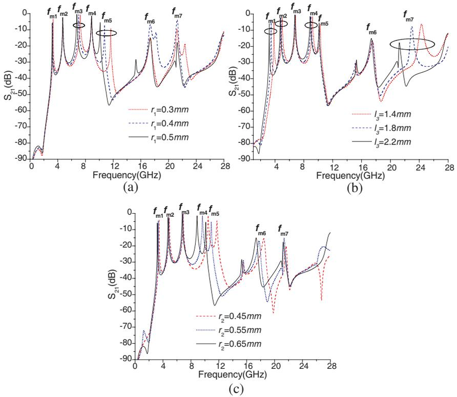
**Figure 2.** Simulated  $S_{21}$ -magnitude of weak coupling stub-loaded MMR with  $l_1 = 1.65$  mm,  $l_2 = 4.5$  mm,  $l_4 = 0.2$  mm,  $l_5 = 0.2$  mm,  $w_1 = w_2 = 0.1$  mm, strip\_w = 0.1 mm, gap\_w = 0.05 mm. (a) With fixed  $l_3 = 2.2$  mm,  $r_2 = 0.65$  mm and varied  $r_1$ . (b) With fixed  $l_3 = 2.2$  mm,  $r_2 = 0.65$  mm and varied  $l_3$ . (c) With fixed  $l_3 = 2.2$  mm,  $r_2 = 0.65$  mm and varied  $r_2$ .
