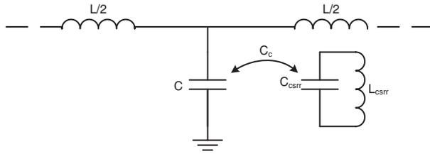
**Figure 2.** Equivalent circuit model of basic CSRR-loaded microstrip line.
