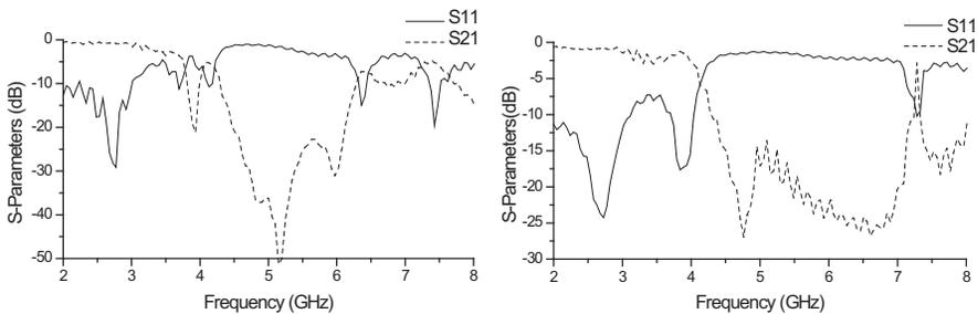
**Figure 4.** Measured  $S$ -parameters of fabricated prototypes, D-II on left and D-III on right side.
