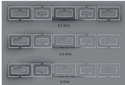
**Figure 5.** Simulated surface current distribution at different frequencies of D-III.
