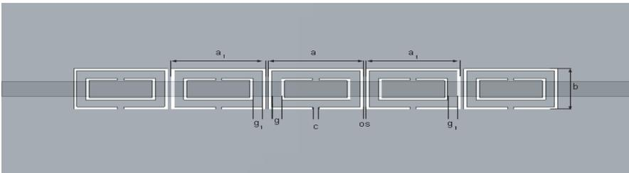
**Figure 1.** Schematics of the CSRR structures etched on the ground plane. The variables  $a_1$  and  $g_1$  are for design D-III, where the adjacent CSRR units are of different size.
