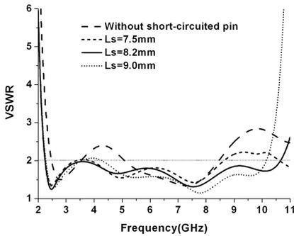
**Figure 2.** Effects of the short-circuited pin on the impedance matching characteristic.
