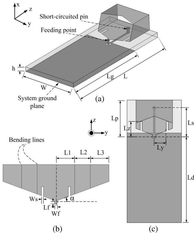
**Figure 1.** (a) Configuration of the proposed internal antenna mounted on the PCB of a wireless USB dongle. (b) Detailed dimensions of the unfolded internal antenna. (c) Top view of the proposed antenna.
