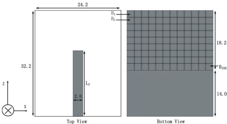
**Figure 1.** Geometry of the proposed UWB antenna.
