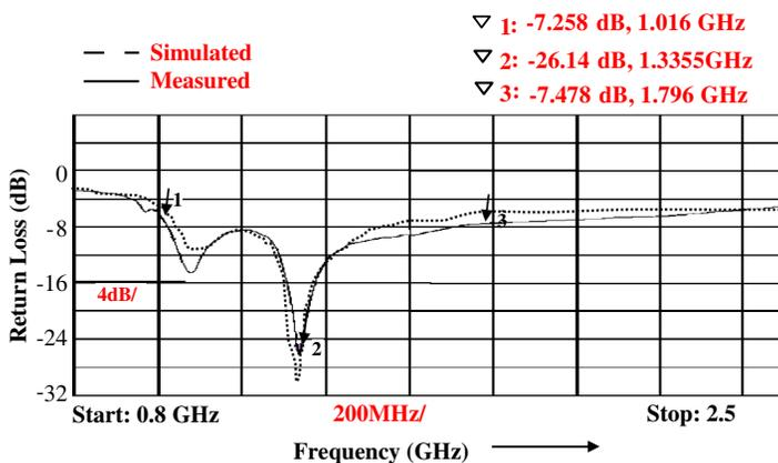
Figure 5. Comparison of Simulated and Measured return loss of the L-band patch antenna.
