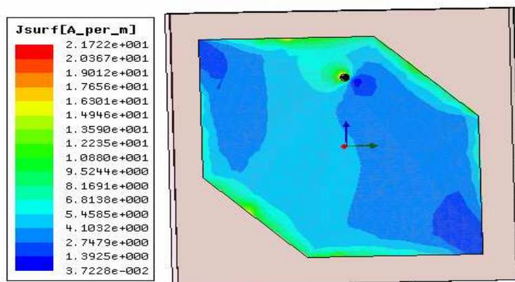
**Figure 2.** Surface current distribution on microstrip at 1.2 GHz.
