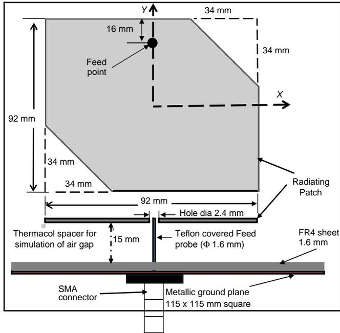
**Figure 1.** Schematic of the proposed broadband circularly polarized patch antenna.
