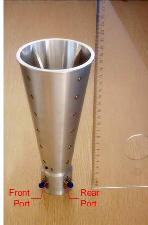
**Figure 7.** Photograph of the manufactured antenna.
