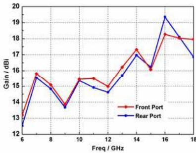
**Figure 10.** Measured gain of the horn antenna.
