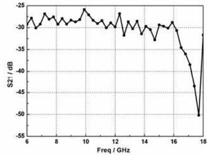
**Figure 9.** Measured isolation of the horn antenna.
