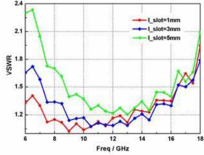
**Figure 4.** Simulated VSWR with various  $l_{slot}$ .
