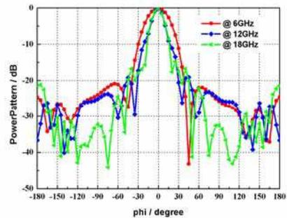
**Figure 11.** Measured  $E$ -plane radiation pattern of the horn antenna.
