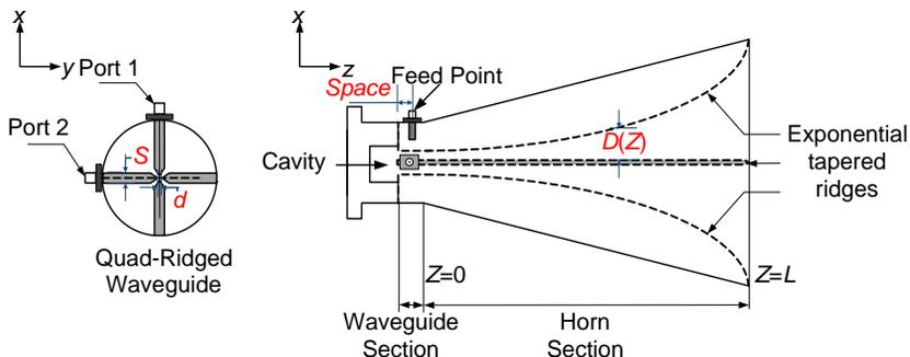
**Figure 1.** Configuration of dual-linear-polarized horn antenna.
