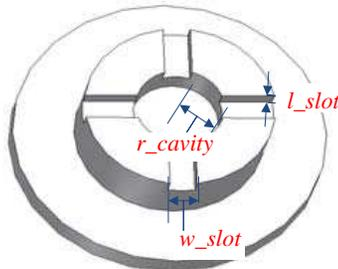
**Figure 2.** Modified shorting cavity structure.
