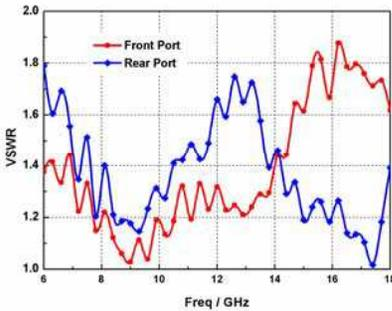
**Figure 8.** Measured VSWR of the horn antenna.
