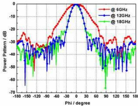
**Figure 12.** Measured  $H$ -plane radiation pattern of the horn antenna.
