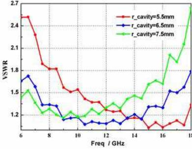
**Figure 3.** Simulated VSWR with various  $r_{cavity}$ .
