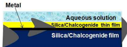
Figure 2. Schematic configuration for four layer SMChA, SMSA, ChMChA and ChMSA sensors.
