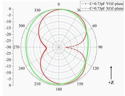
**Figure 9.** The  $E$ - and  $H$ -plane radiation pattern at 3.46 GHz.
