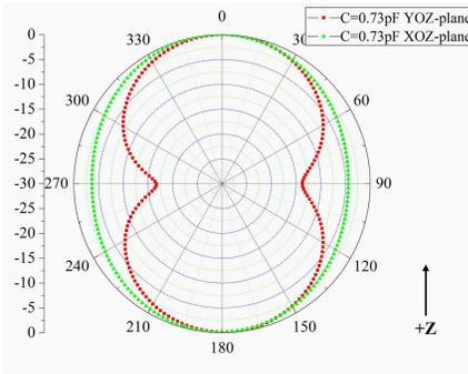
**Figure 8.** The  $E$ - and  $H$ -plane radiation pattern at 2.56 GHz.
