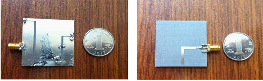
**Figure 2.** Prototypes of the fabricated antenna.
