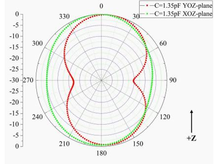
**Figure 7.** The  $E$ - and  $H$ -plane radiation pattern at 3.15 GHz.
