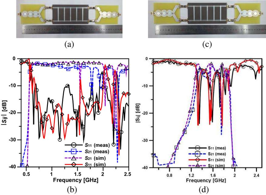
**Figure 6.** Bandpass filter with five-symmetric CRLH unit-cells. (a) Measurement configuration for differential-mode. (b) Measured  $S$ -parameters under differential-mode excitation. (c) Measurement configuration for common-mode. (d) Measured  $S$ -parameters under common-mode excitation.
