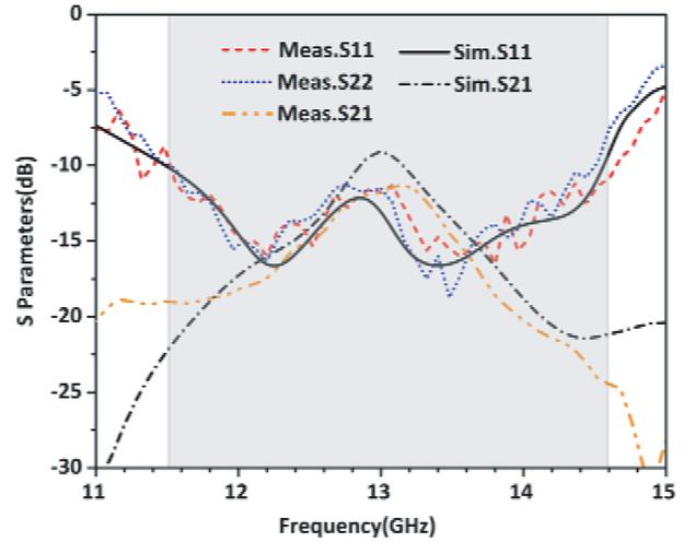
**Figure 5.** Measured and simulated  $S$  parameter.
