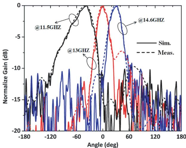
**Figure 6.** Measured and simulated normalized radiation patterns.
